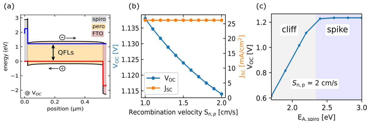
**Fig. 4** (a) Simulated band diagram of the perovskite solar cell used in this study. The diagram shown was acquired at  $V_{OC}$ . (b) Simulated  $V_{OC}$  versus surface recombination velocity at the perovskite/Spiro-OMeTAD interface (blue). The  $J_{SC}$  is not impacted by the variation. (c)  $V_{OC}$  as a function of the Spiro-OMeTAD electron affinity, for a constant interface recombination velocity.
