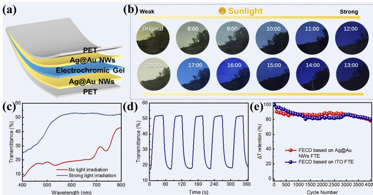
**Fig. 2** (a) Schematic illustration of the PECD; (b–e) characterization of a self-powered EC system based on Ag@Au NWs. Reproduced with permission.<sup>80</sup> Copyright 2022 Elsevier.
