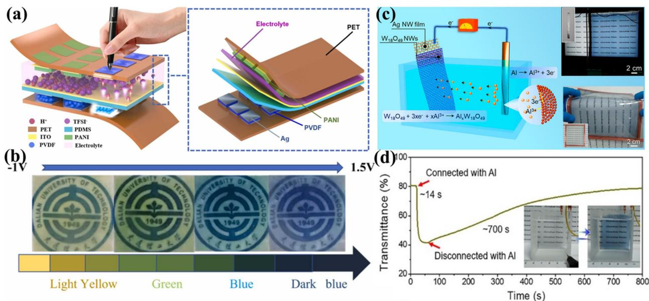
**Fig. 3** (a) Schematic illustration of the PENG-driven tactile display; (b) the color variance under different applied voltages. Reproduced with permission.<sup>82</sup> Copyright 2022 Elsevier Ltd. (c and d) Schematic illustration and characterization of the self-powered flexible EC galvanic cell. Reproduced with permission.<sup>85</sup> Copyright 2021 American Chemical Society.
