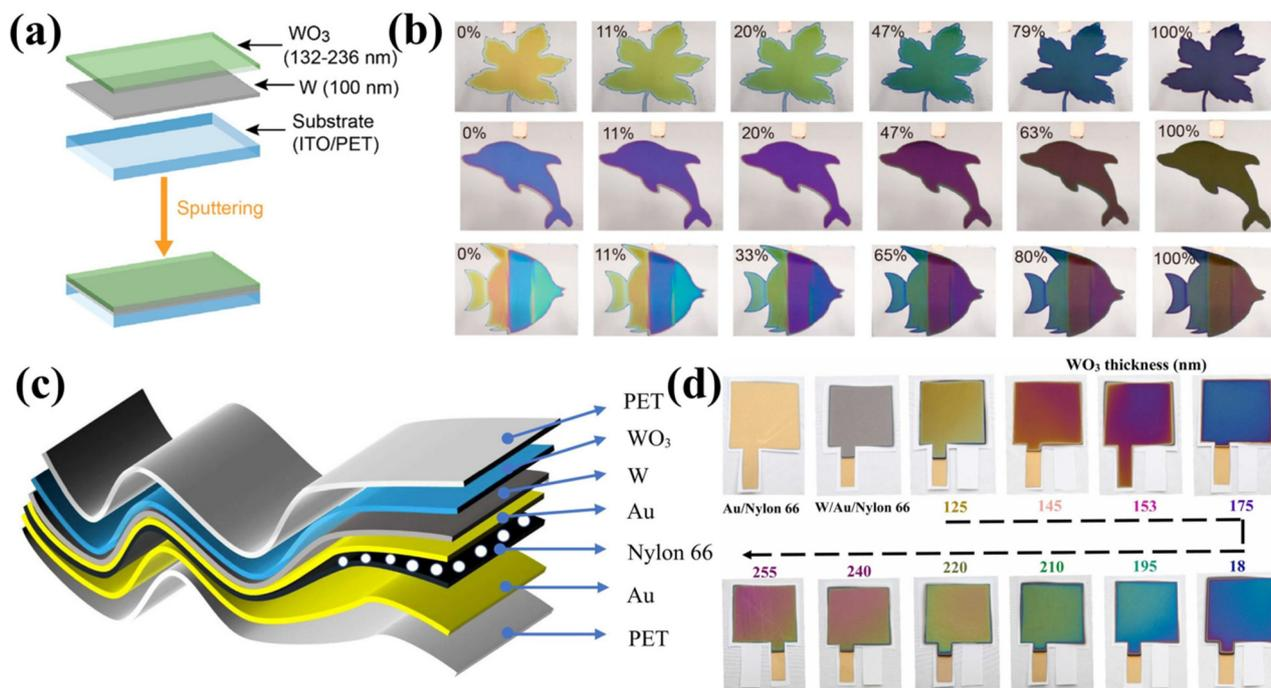
**Fig. 7** (a) Preparation and mechanism of the F–P cavity-type electrochromic supercapacitor electrodes; (b) full-device fabrication with fantastic patterns. Reproduced with permission.<sup>143</sup> Copyright 2020 American Chemical Society. (c) Schematic structure of M-ECD; (d) corresponding optical images of devices with  $\text{WO}_3$  layers of different thicknesses. Reproduced with permission.<sup>142</sup> Copyright 2023 Elsevier B.V.
