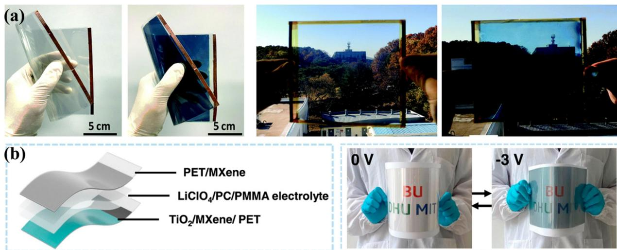
**Fig. 8** (a) Photograph images of a flexible EC smart window. Reproduced with permission.<sup>150</sup> Copyright 2021 Royal Society of Chemistry. (b) Schematic diagram and large-area applications (about 20 × 30 cm) of the flexible solid ECD. Reproduced with permission.<sup>151</sup> Copyright 2021 Springer Nature.
