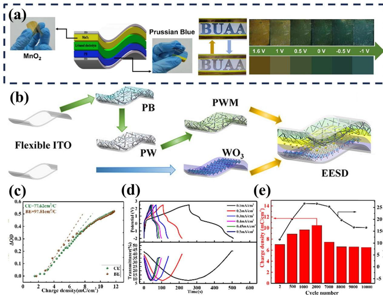
Fig. 6 (a) Schematic diagram of the flexible M-ECD and real photos (up) and emulation images (down) at different voltages. Reproduced with permission.<sup>133</sup> Copyright 2023 American Chemical Society. Schematic illustration (b) and relevant characterizations (c–e) of the present EESD. Reproduced with permission. Copyright 2022 American Chemical Society.
