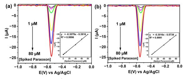
Fig. 7 Voltammograms at a scan rate of 50 mV s<sup>-1</sup> using Ti<sub>3</sub>C<sub>2</sub>T<sub>x</sub>/MWCNT-OH from measurements in pH 8 phosphate buffer at various concentrations of paraoxon-ethyl ranging from 1 to 80 μM in samples (a) green grapes and (b) red grapes.
