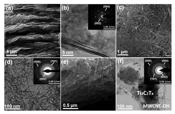
Fig. 3 FESEM and HRTEM images (insets: SAED analysis) of (a and b) Ti<sub>3</sub>C<sub>2</sub>T<sub>x</sub>, (c and d) MWCNT-OH, and (e and f) Ti<sub>3</sub>C<sub>2</sub>T<sub>x</sub>/MWCNT-OH nanocomposite, respectively.
