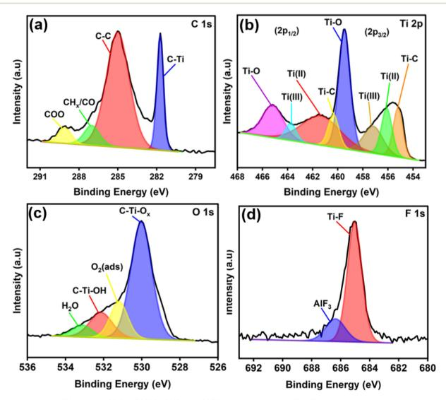
Fig. 2 High resolution XPS spectra of (a) C 1s, (b) Ti 2p, (c) O 1s, and (d) F 1s of the as-prepared  $Ti_3C_2T_x$ .
