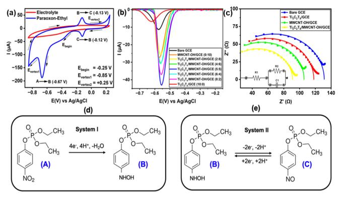
Fig. 4 (a) Cyclic voltammogram of 100  $\mu$ M paraoxon-ethyl in 0.1 M phosphate buffer solution (PBS) at pH 7.0 using bare GCE; (b) differential pulse voltammogram of paraoxon-ethyl measured using different types of electrodes; (c) Nyquist plot of different type of electrodes using 5 mM K<sub>3</sub>[Fe (CN)<sub>6</sub>]; and the proposed electrochemical redox reaction of paraoxon-ethyl according to (d) system I and (e) system II.
