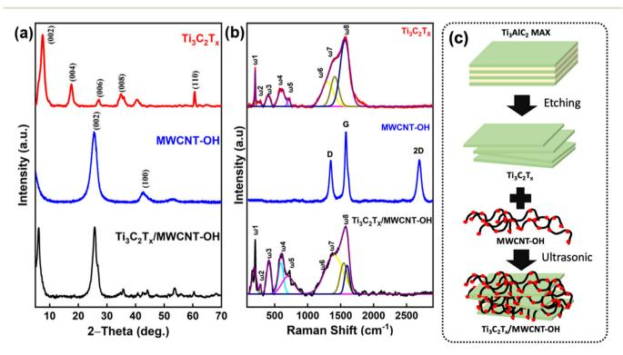
Fig. 1 (a) X-ray diffractogram and (b) Raman spectra of  $Ti_3C_2T_{xx}$ , MWCNT-OH, and  $Ti_3C_2T_{xx}$ /MWCNT-OH nanocomposites; (c) schematic illustration for the formation of nanocomposite.
