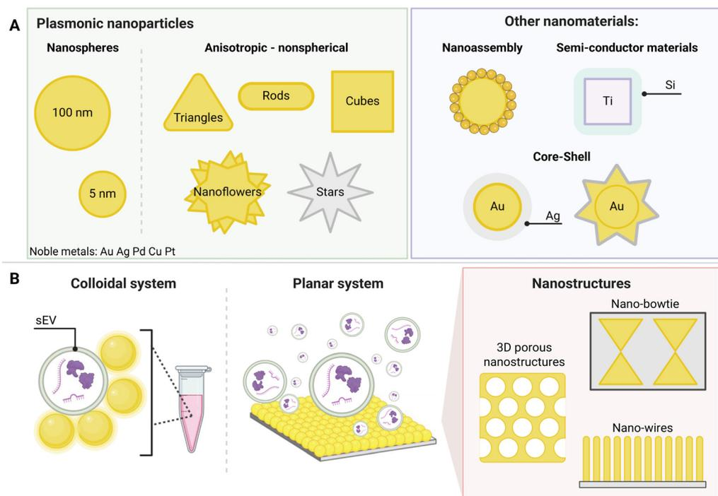
**Fig. 2** SERS substrates depicting (A) plasmonic nanoparticles used for SERS label-free detection and (B) assay structures including both colloidal and planar systems, as well as examples of nanostructures used within planar systems.
