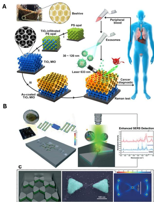
**Fig. 3** Label-free assays with unique nanostructures as SERS substrate. (A) Beehive structure to enhance sEVs Raman fingerprint. Adapted from ref. 48 with permission from ACS Applied Materials and Interfaces, copyright [2021]. (B) Nano-bowtie structures used as SERS substrate for sEVs detection. Adapted from ref. 3 with permission from Lab on a Chip, copyright [2020].
