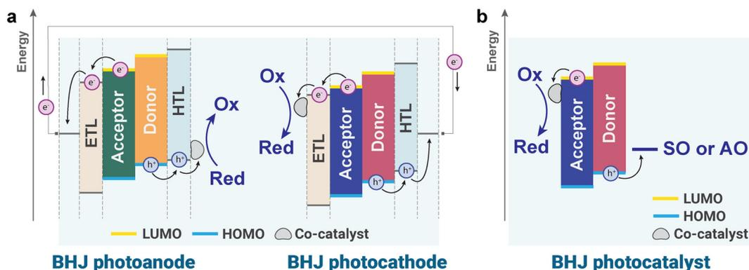
**Fig. 1** Illustration of working mechanisms of (a) BHJ-based PEC cells and (b) BHJ-based PCs. PEC cells consist of a BHJ photocathode for reduction reactions and a BHJ photoanode for oxidation reactions. BHJ PCs typically comprise a single BHJ blend to drive both reduction and oxidation reactions simultaneously. Ox: oxidized species, Red: reduced species, SO: sacrificial oxidation, AO: alternative oxidation.
