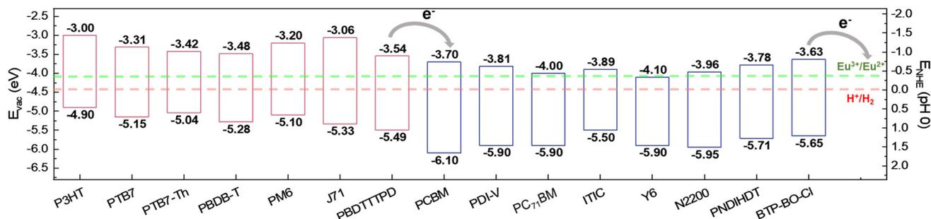
Fig. 3 Energy level alignment of conjugated polymers and small molecules for BHJ photocathodes with redox potential of  $\text{H}^+/\text{H}_2$  at pH 0 and  $\text{Eu}^{3+}/\text{Eu}^{2+}$  (sacrificial agent).
