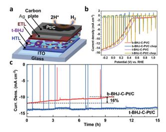
Fig. 9 (a) Schematic diagram of the carbon-encapsulated ternary BHJ (PBDB-T:ITIC:PC71BM) photocathode with PEDOT:PSS and PDNIO as HTL and ETL, respectively. (b) The J-V curves and (c) CA curves of the b-BHJ (PBDB-T:ITIC)-C-Pt/C and t-BHJ-C-Pt/C photocathodes in 0.1 M  $H_2SO_4$  solution (pH 1.0) at 0  $V_{RHE}$  under AM 1.5 G illumination. Adapted with permission. 48 Copyright 2022, Wiley-VCH GmbH.
