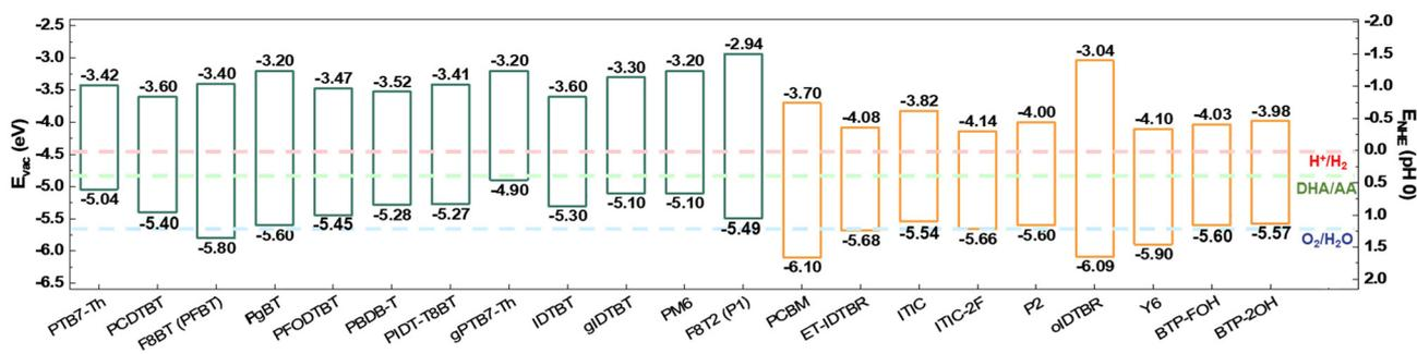
Fig. 22 Energy level alignment of conjugated polymers and small molecules for photocatalysts with redox potential of  $H^+/H_2$ , DHA/AA, and  $O_2/H_2O$ .
