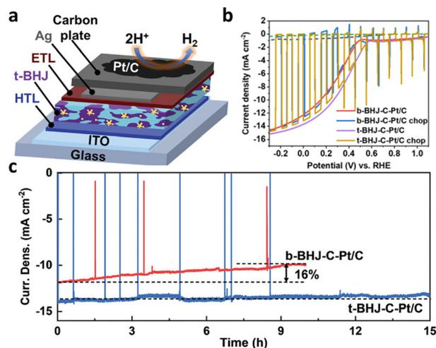
**Fig. 9** (a) Schematic diagram of the carbon-encapsulated ternary BHJ (PBDB-T:ITIC:PC<sub>71</sub>BM) photocathode with PEDOT:PSS and PDNIO as HTL and ETL, respectively. (b) The  $J$ - $V$  curves and (c) CA curves of the b-BHJ (PBDB-T:ITIC)-C-Pt/C and t-BHJ-C-Pt/C photocathodes in  $0.1 \text{ M H}_2\text{SO}_4$  solution (pH 1.0) at  $0 \text{ V}_{\text{RHE}}$  under AM 1.5 G illumination. Adapted with permission.<sup>48</sup> Copyright 2022, Wiley-VCH GmbH.
