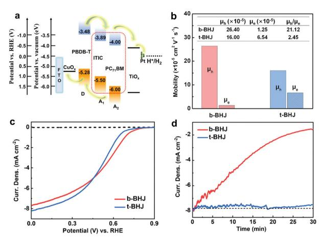
Fig. 5 (a) Energy level diagram of PBDB-T, ITIC, and PC<sub>71</sub>BM in ternary photocathode. (b)  $\mu_h$  and  $\mu_e$  of the binary BHJ without PC<sub>71</sub>BM and ternary BHJ with PC<sub>71</sub>BM films. (c) J-V curves of the binary and ternary BHJ-based photocathode under 1 sun illumination in 0.1 M H<sub>2</sub>SO<sub>4</sub> (pH = 1.0). (d) CA tests at 0 V<sub>RHF</sub> for the binary and ternary BHJ-based photocathode. Adapted with permission. 48 Copyright 2022, Wiley-VCH GmbH.
