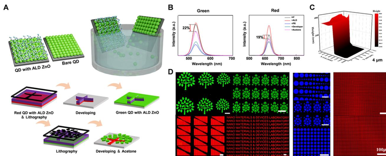
**Fig. 8** (A) Schematic of the photolithographic patterning of ZnO-passivated InP QDs. (B) Intensity of green and red QDs during the patterning processes. (C) Height profile of the patterned QD microstructure. (D) Fluorescence images of the red and green InP QDs and blue ZnSeTe QD patterns. Reprinted with permission from ref. 31. Copyright 2023, American Chemical Society.
