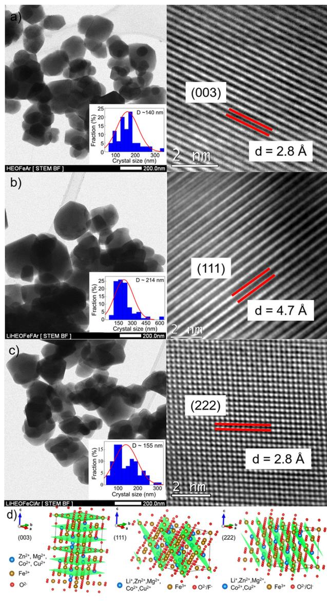
**Fig. 2** (S)TEM and HR-TEM micrographs of (a) HEOFe, (b) LiHEOFef, and (c) LiHEOFelCl synthesized samples. Insets show the particle size distribution. Interplanar distances,  $d$ , correspond to those determined from eqn (5). (d) Idealized spinel structure of the investigated samples. Particular crystal planes for HEOFe (003), LiHEOFef (111), and LiHEOFelCl (222) are highlighted.
