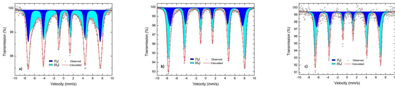
**Fig. 4** The room-temperature  $^{57}\text{Fe}$  Mössbauer spectra of (a) HEOFe, (b) LiHEOFef, and (c) LiHEOFefCl. The dark blue and light blue spectra correspond to tetrahedrally ( $T_d$ ) and octahedrally ( $O_h$ ) coordinated iron cations, respectively.
