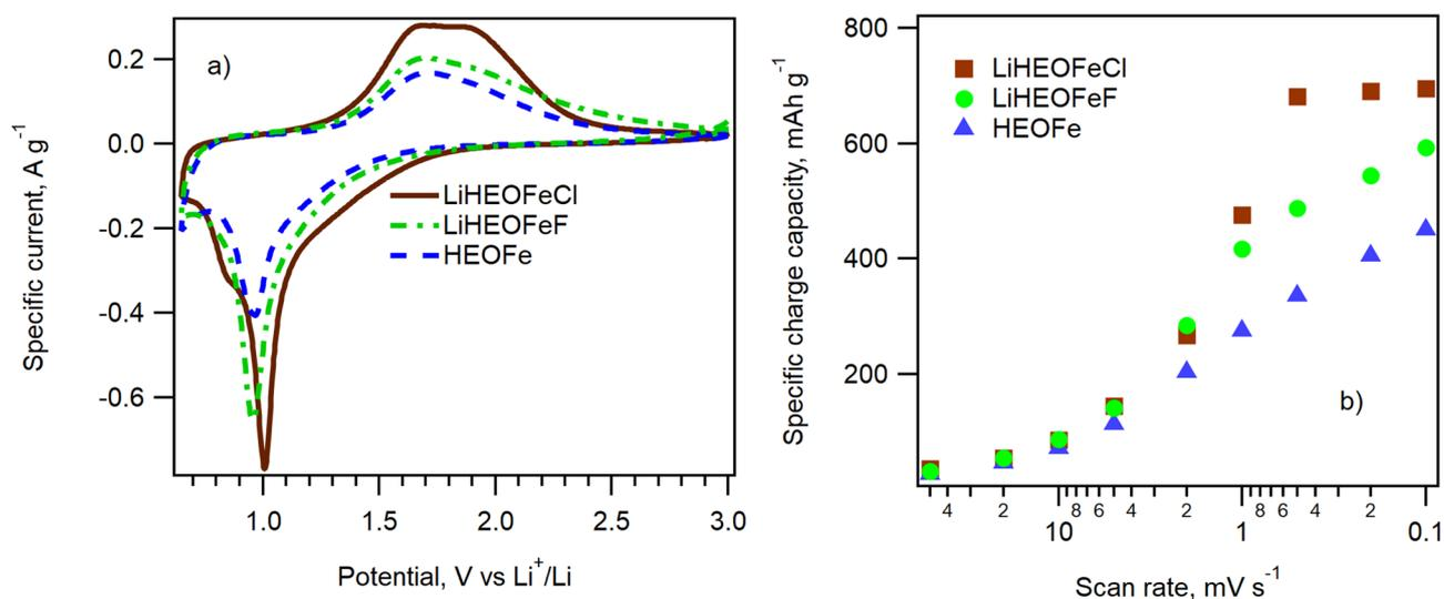
**Fig. 6** (a) Cyclic voltammograms measured on 2032-coin cells containing LiHEOFeCl, LiHEOFeF, and HEOFe with a scan rate of 0.1 mV s<sup>-1</sup>. (b) The scan-rate dependence of the charge capacities calculated from the discharge branch of the cyclic voltammogram on the scan rate for HEOFe (blue triangles), LiHEOFeCl (brown squares), and LiHEOFeF (green circles).
