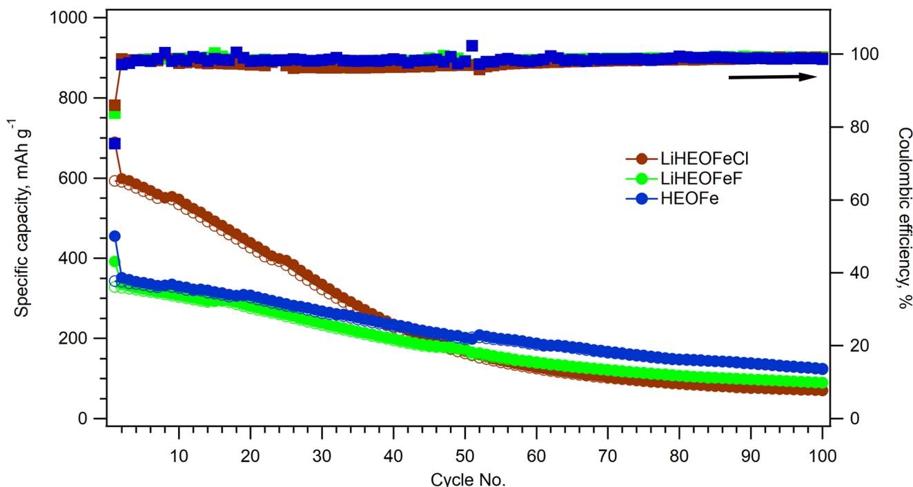
Fig. 7 Galvanostatic chronopotentiometry at 1C rate for HFeOFe (blue circles), LiHFeOFeCl (brown circles), and LiHFeOFeF (green circles). The charge capacity within charging is marked with full circles and the charging capacity within discharging with empty circles. The corresponding coulombic efficiencies for HFeOFe, LiHFeOFeCl, and LiHFeOFeF are depicted by squares of the same color coding.
