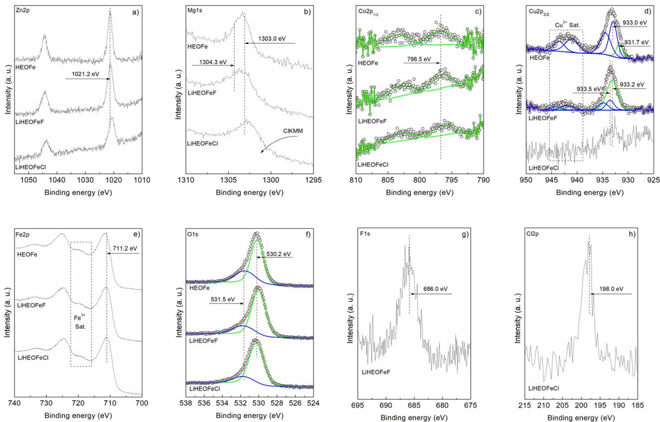
**Fig. 5** High-resolution XPS spectra of the HEOFe, LiHEOFef, and LiHEOFefCl compounds showing the signals corresponding to (a) Zn 2p, (b) Mg 1s, (c) Co 2p<sub>1/2</sub>, (d) Cu 2p<sub>3/2</sub>, (e) Fe 2p, (f) O 1s, (g) F 1s and (h) Cl 2p.
