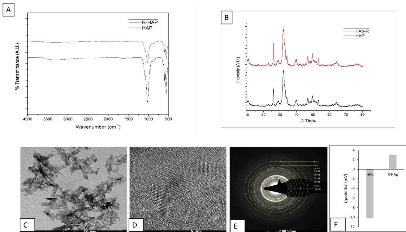
**Fig. 1** Characterization of R-HAp nanoparticles. (A) FTIR spectrum of R-HAp and HAp Np. (B) XRD spectrum of R-HAp and HAp Np. (C) TEM and (D) HR-TEM micrographs and (E) SAED pattern. (F)  $\zeta$ -Potential measurements of R-HAp Nps, compared with un-functionalized HAp NPs.
