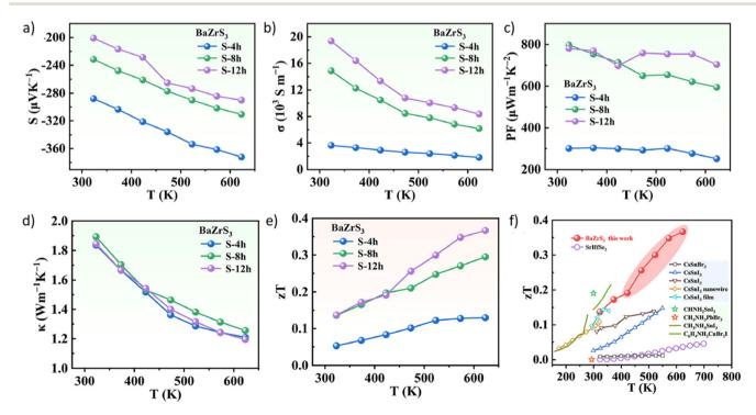
Fig. 30 Thermoelectric performance of BaZrS<sub>3</sub>. (a)–(f) Seebeck coefficient (S), electrical conductivity (σ), power factor (PF), thermal conductivity (k), and thermoelectric efficiency (zT) as functions of annealing temperature for dense BaZrS<sub>3</sub> bulk samples. (a)–(f) Reproduced with permission. Copyright 2024, Elsevier.
