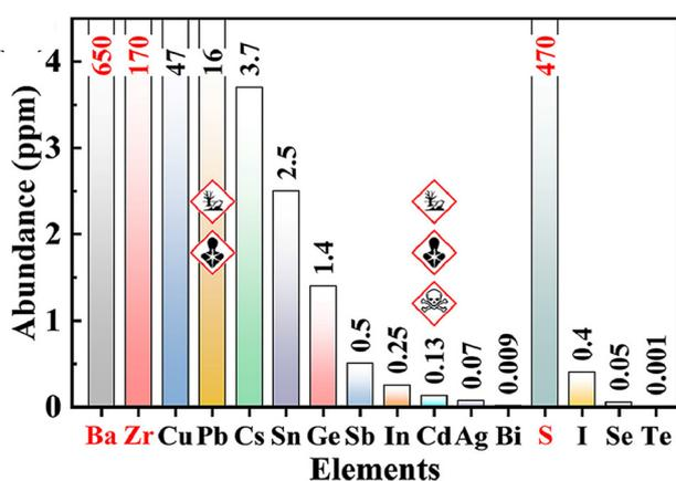
Fig. 3 Schematic illustrating the relative abundance of Ba, Zr, and S in comparison to other key elements utilized in thin-film photovoltaic applications. Reproduced with permission.<sup>66</sup> Copyright 2024, Elsevier.
