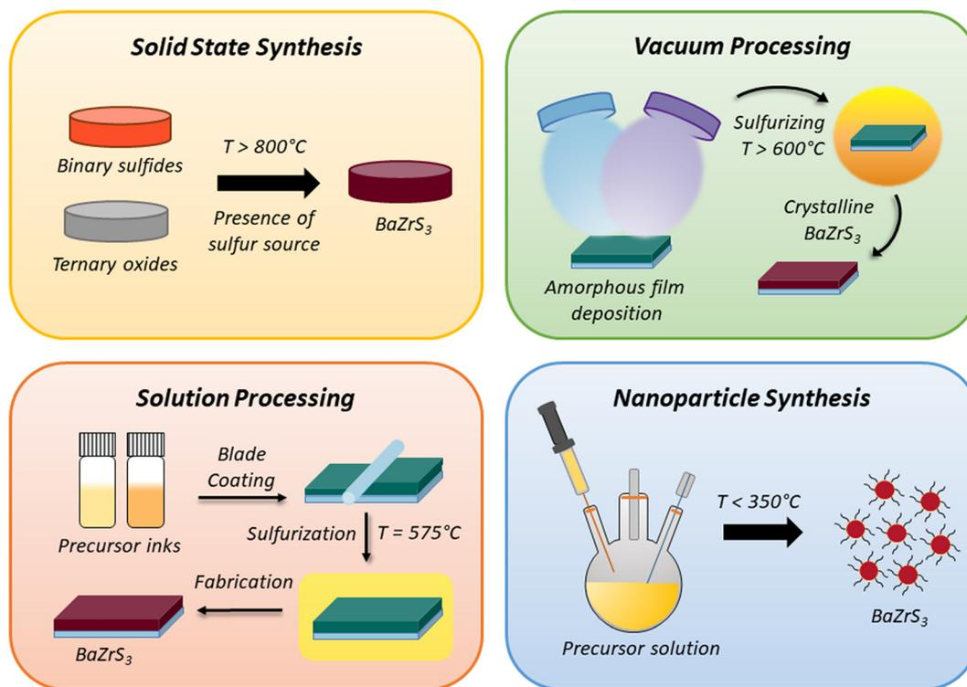
Fig. 6 Schematic illustrating the various synthesis methods used for the preparation of BaZrS<sub>3</sub> and related compounds.
