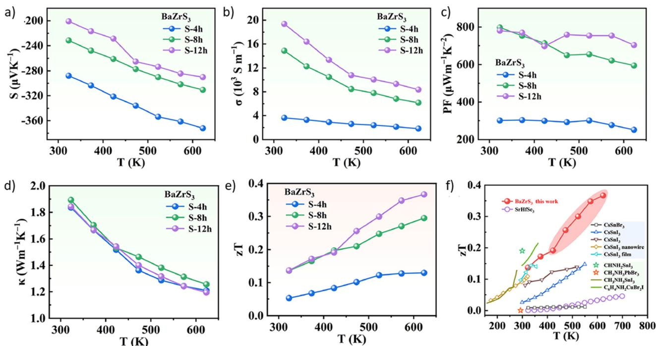
Fig. 30 Thermoelectric performance of BaZrS<sub>3</sub>. (a)–(f) Seebeck coefficient ( $S$ ), electrical conductivity ( $\sigma$ ), power factor (PF), thermal conductivity ( $\kappa$ ), and thermoelectric efficiency ( $zT$ ) as functions of annealing temperature for dense BaZrS<sub>3</sub> bulk samples. (a)–(f) Reproduced with permission.<sup>66</sup> Copyright 2024, Elsevier.
