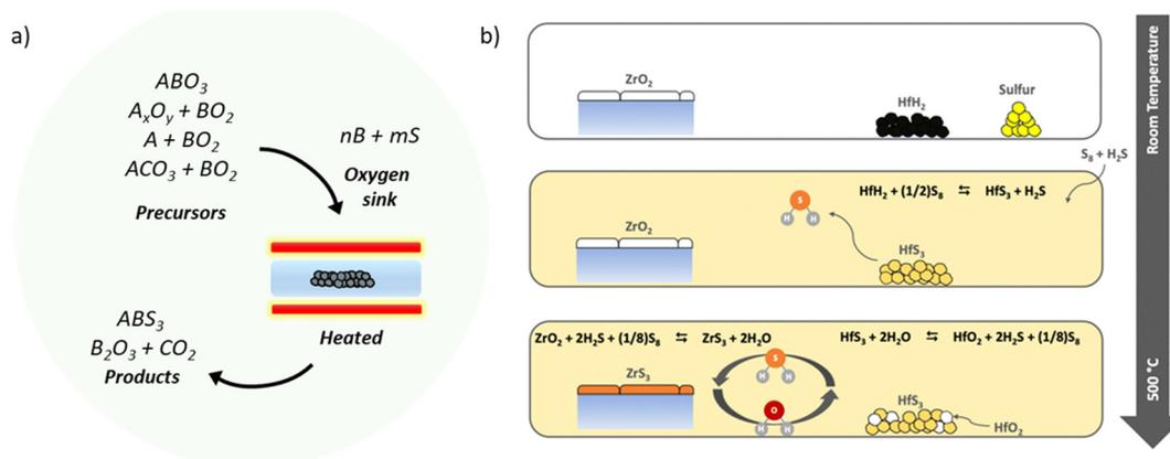
**Fig. 7** (a) Schematic illustrating the conversion of binary and ternary oxide powders into ternary chalcogenides using boron and sulfur. (a) Adapted with permission.<sup>88</sup> (b) Schematic depicting the conversion of  $ZrO_2$  into  $ZrS_3$  using  $HfH_2$  and sulfur. (b) Reproduced with permission.<sup>73</sup> Copyright 2023, Royal Society of Chemistry.
