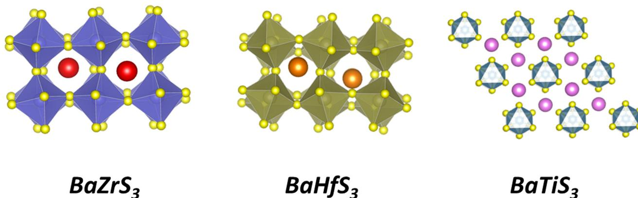
**Fig. 1** Crystal structures of BaZrS<sub>3</sub>, BaHfS<sub>3</sub>, and BaTiS<sub>3</sub>. BaZrS<sub>3</sub> and BaHfS<sub>3</sub> exhibit distorted perovskite structures, while BaTiS<sub>3</sub> adopts a hexagonal crystal structure.
