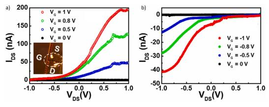
Fig. 28 The drain-source current (I<sub>DS</sub>) versus drain-source voltage (V<sub>DS</sub>) for the FET fabricated using the film annealed at 650 °C under (a) positive and (b) negative gate voltages ( $V_G$ ). (a) and (b) Reproduced with permission. <sup>93</sup> Copyright 2021, American Chemical Society.
