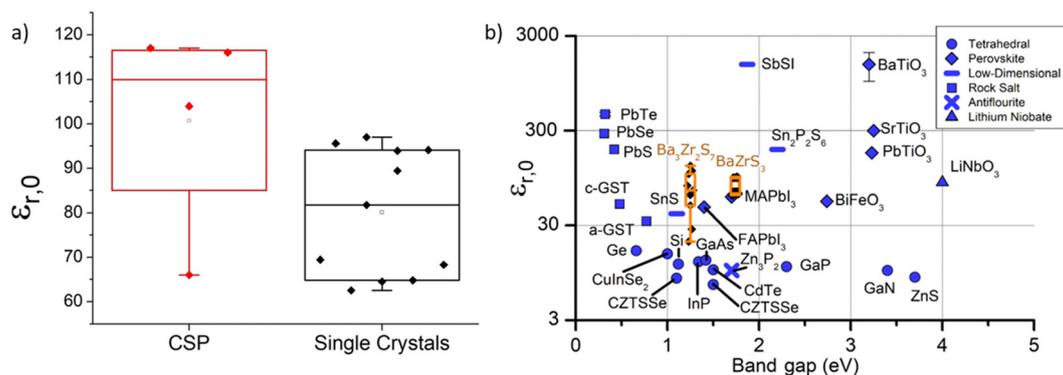
**Fig. 4** Dielectric constant of BaZrS<sub>3</sub> and other inorganic materials. (a) Comparison of the dielectric constant for densified BaZrS<sub>3</sub> obtained through cold-sintering and single crystal BaZrS<sub>3</sub>. (b) Plot illustrating the relationship between the dielectric constant and bandgap for various inorganic materials. (a) and (b) Reproduced with permission.<sup>69</sup> Copyright 2021, Springer Nature.
