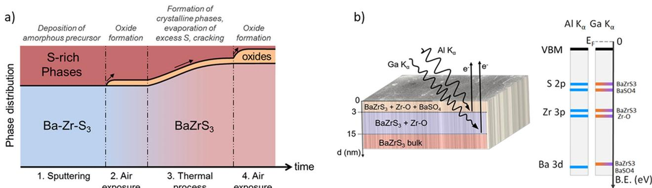
**Fig. 17** Surface oxide impurities in BaZrS<sub>3</sub>. (a) Schematic representation of phase distribution in the BaZrS<sub>3</sub> film over time upon exposure to air. (a) Reproduced with permission.<sup>97</sup> Copyright 2020, American Chemical Society. (b) Schematic illustrating the different phases present in the near-surface layers, as identified by hard X-ray photoelectron spectroscopy. (b) Reproduced with permission.<sup>139</sup> Copyright 2024, American Chemical Society.
