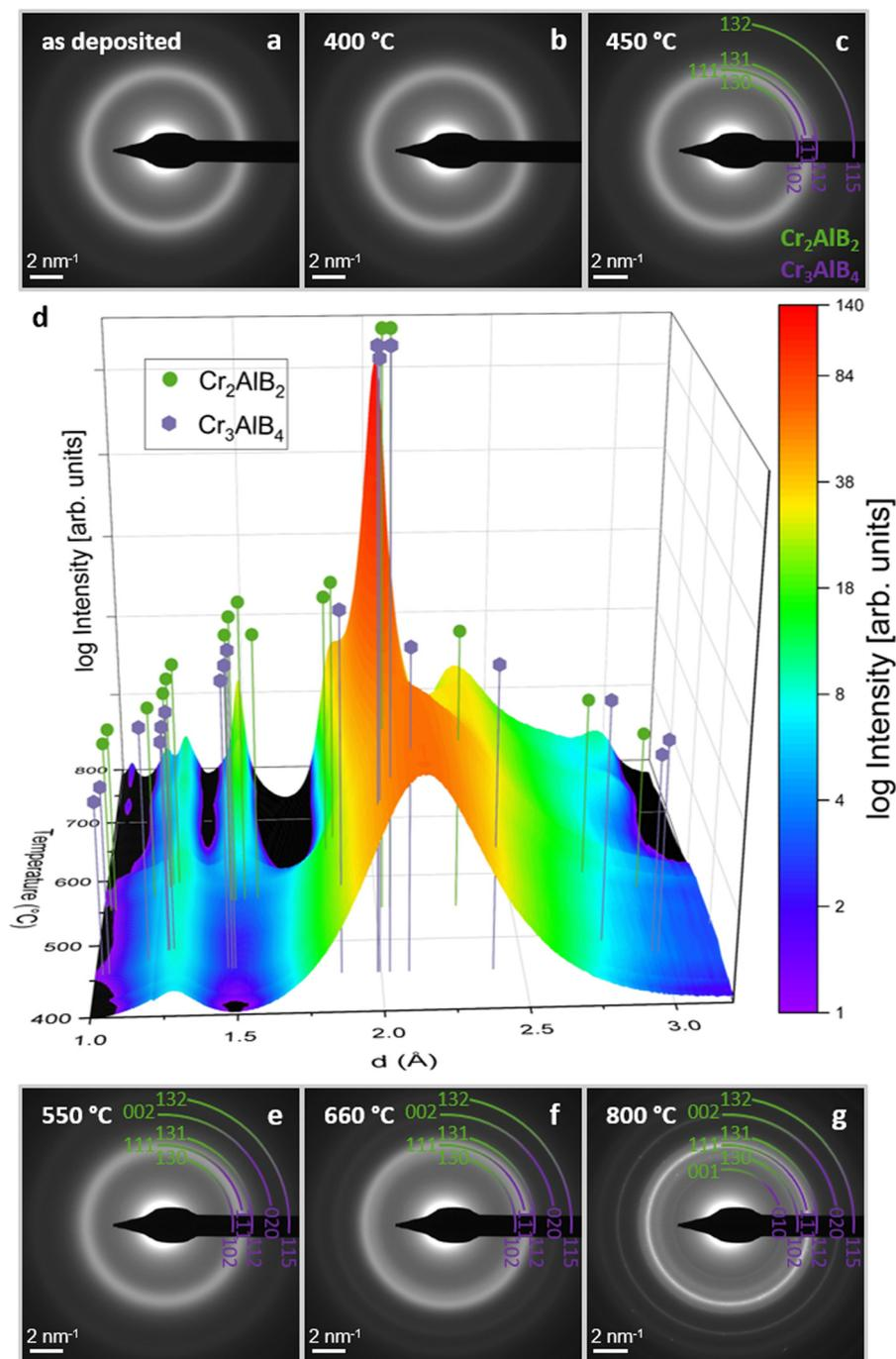
**Fig. 3** In situ SAED patterns (a–c and e–g) and the corresponding integrated intensity plotted with respect to temperature (d). Peak positions of  $\text{Cr}_2\text{AlB}_2$  and  $\text{Cr}_3\text{AlB}_4$  are indicated. A first transformation is visible at 450 °C (see ESI S5†) with subsequent emergence of peaks corresponding to  $\text{Cr}_2\text{AlB}_2$  and  $\text{Cr}_3\text{AlB}_4$ .
