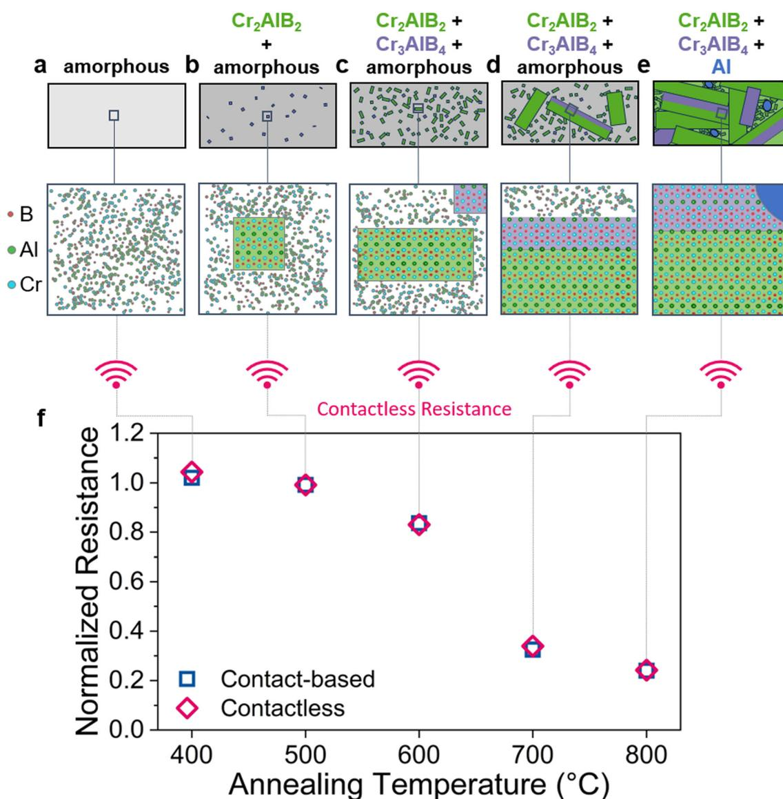
**Fig. 1** Schematic illustration of crystal structure and grain size after annealing (a–e). Contact-based and contactless measured, normalized resistance versus annealing temperature (f) showing a crystal structure and grain size dependent resistivity decrease with increasing annealing temperature. Resistance data are normalized with respect to their initial value before annealing.
