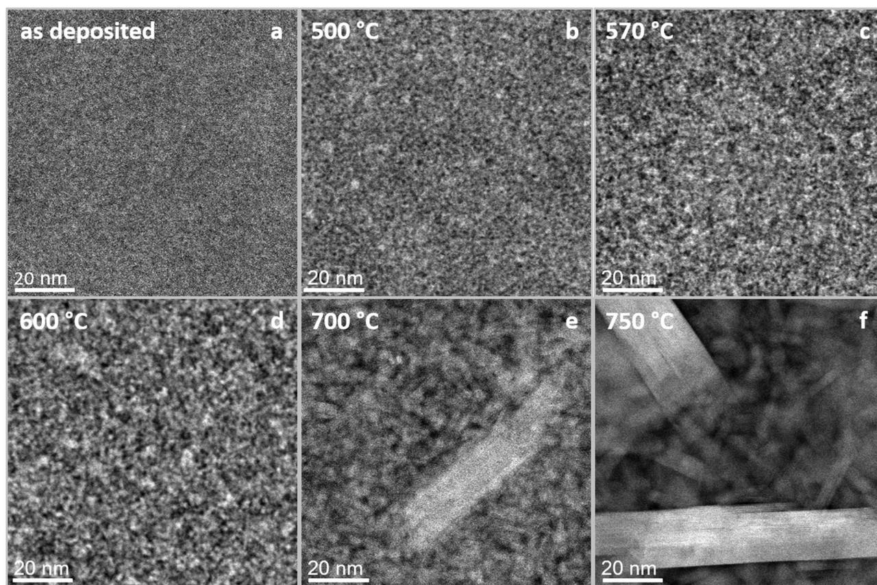
Fig. 4 HRSTEM micrographs taken during *in situ* annealing at indicated temperatures (a–f). The amorphous as deposited structure becomes partly crystalline after 500 °C, whereby MAB phase formation is observed, with a significant increase in crystal domain size after 700 °C.
