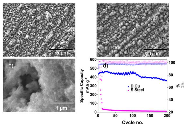
**Fig. 4** (a) DCu before PVD (b) pristine SnSb coated DCu anode & (c) SEM imaging of SnSb coated DCu post-mortem after charge and discharge cycling vs.  $\text{Na}/\text{Na}^+$ . (d) Increased mass loading SnSb on SS and DCu galvanostatic cycling data vs.  $\text{Na}/\text{Na}^+$  at  $250 \text{ mA h g}^{-1}$ .
