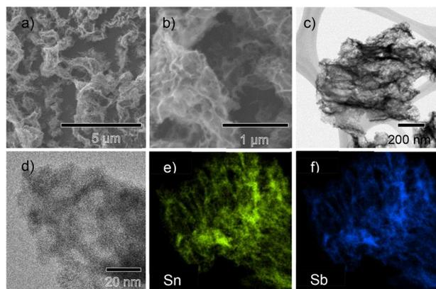
**Fig. 3** (a) & (b) SEM imaging of SnSb after 100 galvanostatic cycles vs.  $\text{Na}/\text{Na}^+$ . (c) & (d) TEM and HRTEM imaging of SnSb after extended galvanostatic cycling vs.  $\text{Na}/\text{Na}^+$ . (e) & (f) EDX mapping of Sn and Sb respectively.
