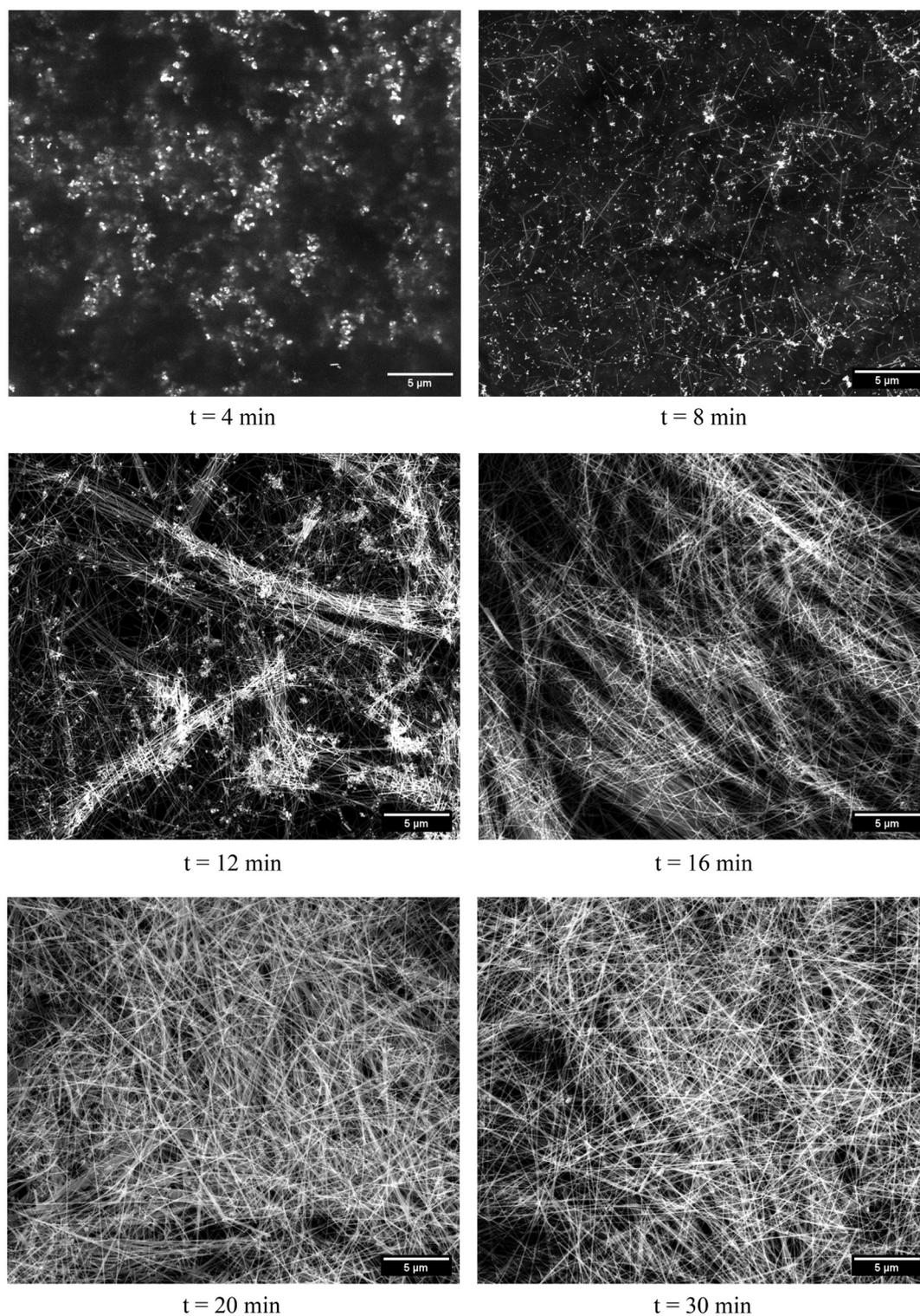
**Fig. 8** SEM images taken at six different residence times in the millifluidic reactor. Nucleation occurs at  $t = 4$  min, AgNWs are beginning to form at  $t = 8$  min, and the wires continue to grow from  $t = 12$  min through  $t = 30$  min. (Scale Bars:  $5 \mu\text{m}$ ).
