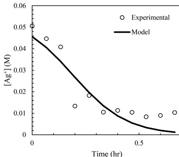
Fig. 10 Non-linear fit of experimental  $[\text{Ag}^+]$  as a function of residence time in the MFR.
