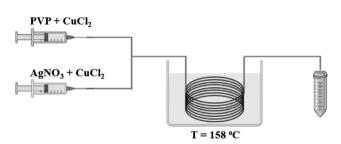
Fig. 3 Schematic of the MFR configuration for the polyol AgNW synthesis.
