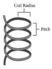
Fig. 12 The radius of the reactor tubing, r, and the pitch (space between coils), p, is considered when calculating the critical radius for the He.
