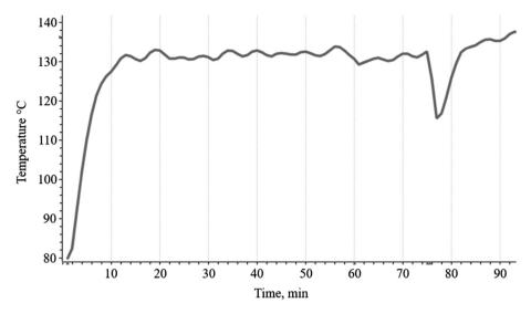
Fig. 11 Temperature profile taken for the batch reactor using in situ react IR.
