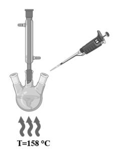
Fig. 2 Schematic of the batch reactor setup for the polyol AgNW synthesis
