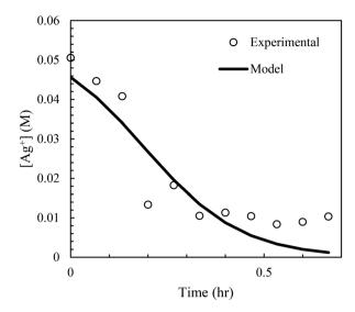
Fig. 10 Non-linear fit of experimental [Ag+] as a function of residence time in the MFR.
