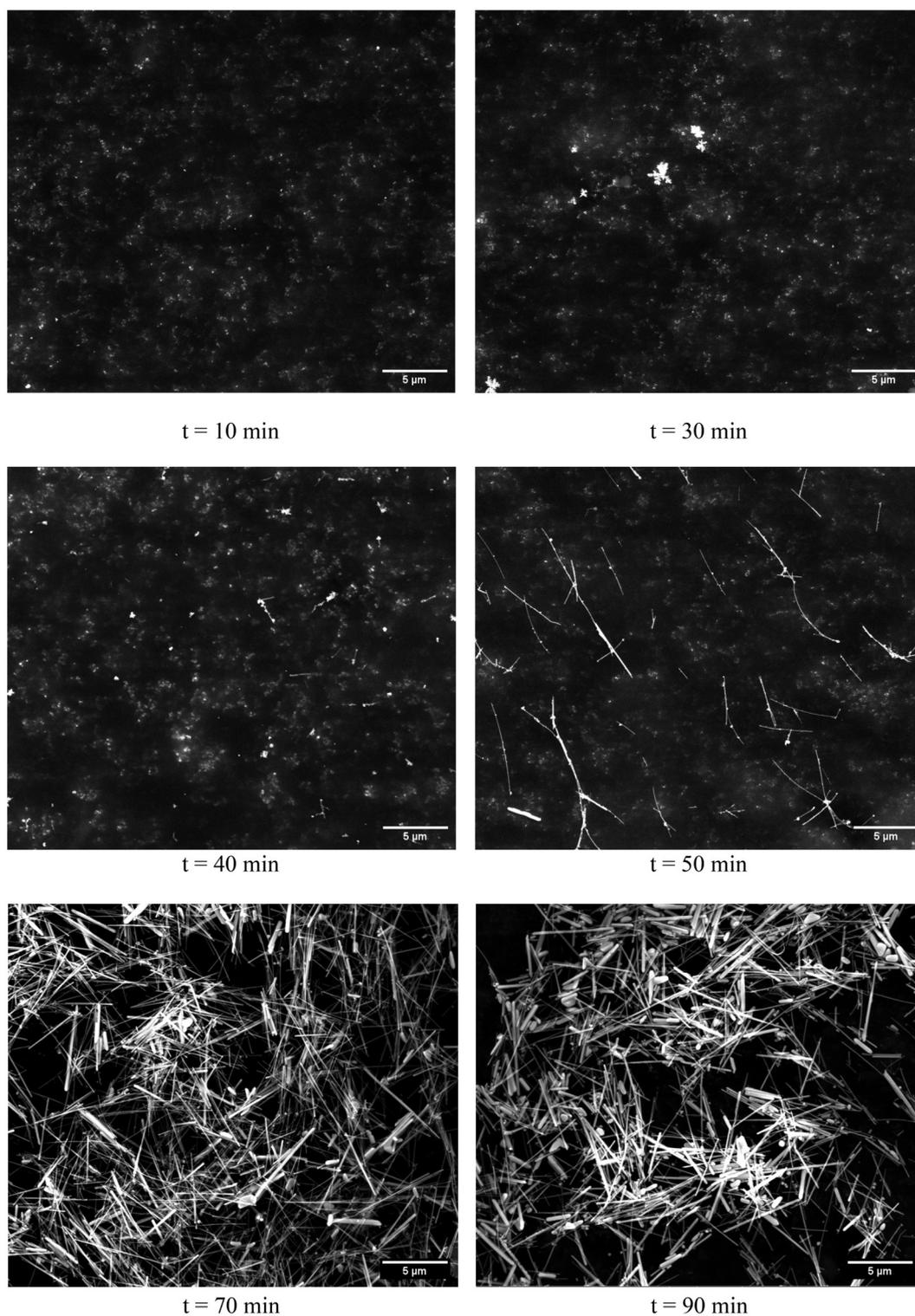
Fig. 7 SEM images taken at six different reaction times in the batch reactor. Nucleation begins at  $t = 10$  min, AgNWs are beginning to form at  $t = 40$  min, and the wires continue growing from  $t = 50$  min through  $t = 90$  min. (Scale bars:  $5 \mu\text{m}$ ).
