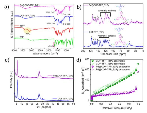
Fig. 2 (a) FT-IR spectra of COF-TFP\_TzPy and Pd@COF-TFP\_TzPy. (b) Solid-state <sup>13</sup>C-NMR spectra of COF-TFP\_TzPy and Pd@COF-TFP\_TzPy (\* indicates side bands). (c) Powder X-ray diffraction patterns of COF-TFP\_TzPy and Pd@COF-TFP\_TzPy. (d) Low-temperature N2 adsorption-desorption isotherm.
