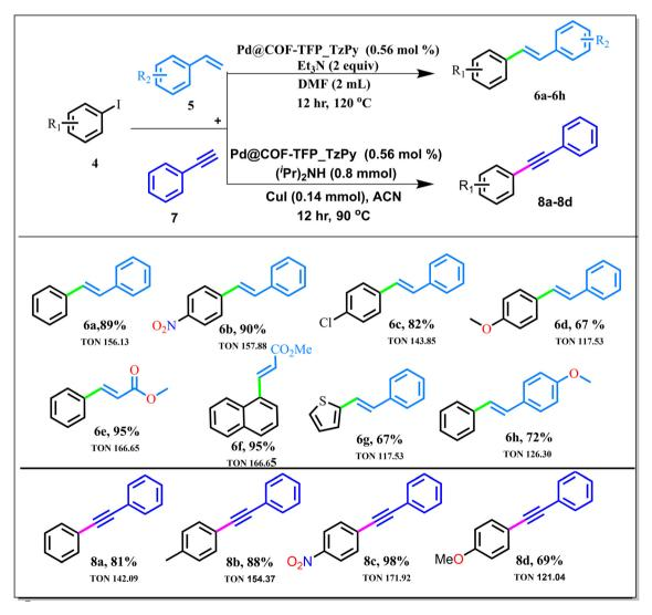
Scheme 4 Substrate scope of Heck and Sonogashira coupling. Reaction conditions: aryl iodide 4 (0.4 mmol), 5 (0.8 mmol), Et<sub>3</sub>N (0.8 mmol), and 5.0 mg (0.56 mol% of Pd@COF-TFP\_TzPy) of catalyst were stirred in 2 ml of DMF for 12 h. Aryl iodide 4 (0.4 mmol), 8 (0.6 mmol), iPr<sub>2</sub>NH (0.8 mmol), Cul (0.14 mmol), and 5.0 mg (0.56 mol% of Pd@COF-TFP\_TzPy) of catalyst were stirred in 4 ml of ACN for 12 h.
