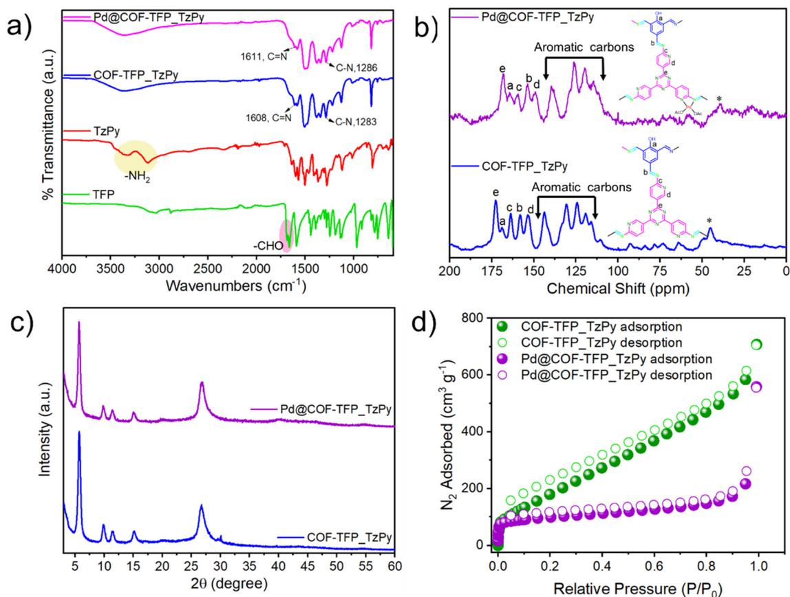
**Fig. 2** (a) FT-IR spectra of COF-TFP\_TzPy and Pd@COF-TFP\_TzPy. (b) Solid-state  $^{13}\text{C}$ -NMR spectra of COF-TFP\_TzPy and Pd@COF-TFP\_TzPy (\* indicates side bands). (c) Powder X-ray diffraction patterns of COF-TFP\_TzPy and Pd@COF-TFP\_TzPy. (d) Low-temperature  $\text{N}_2$  adsorption–desorption isotherm.
