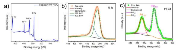
Fig. 5 (a) XPS survey spectra of Pd@COF-TFP\_TzPy. (b) HR-XPS of the N 1s spectrum. (c) HR-XPS of Pd 3d in Pd@COF-TFP\_TzPy.
