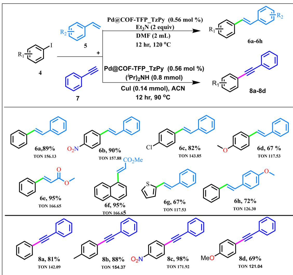
Scheme 4 Substrate scope of Heck and Sonogashira coupling. Reaction conditions: aryl iodide **4** (0.4 mmol), **5** (0.8 mmol), Et<sub>3</sub>N (0.8 mmol), and 5.0 mg (0.56 mol% of Pd@COF-TFP\_TzPy) of catalyst were stirred in 2 ml of DMF for 12 h. Aryl iodide **4** (0.4 mmol), **8** (0.6 mmol), (iPr)<sub>2</sub>NH (0.8 mmol), CuI (0.14 mmol), and 5.0 mg (0.56 mol% of Pd@COF-TFP\_TzPy) of catalyst were stirred in 4 ml of ACN for 12 h.
