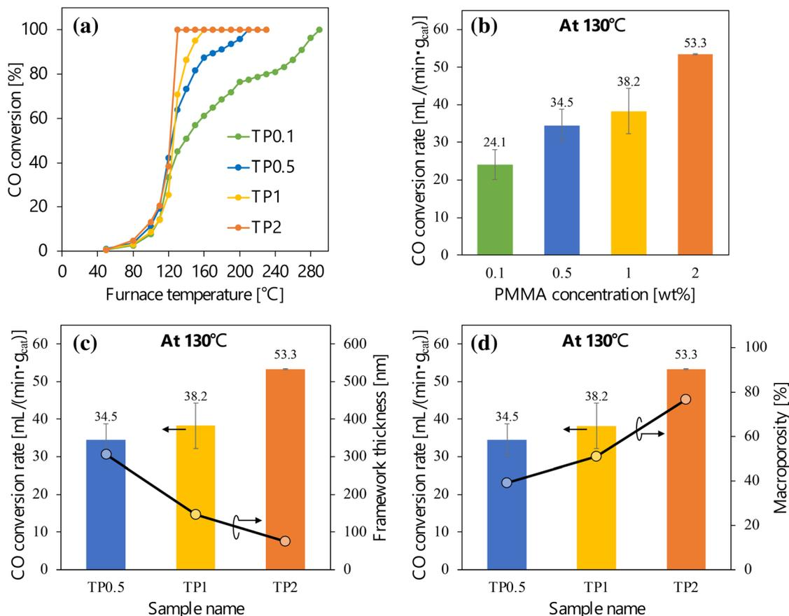
**Fig. 6** (a) CO conversion into CO<sub>2</sub> and (b) CO oxidation rate of porous TWC particles at different PMMA concentrations and its relationship with the (c) framework thickness and (d) macroporosity at 130 °C.
