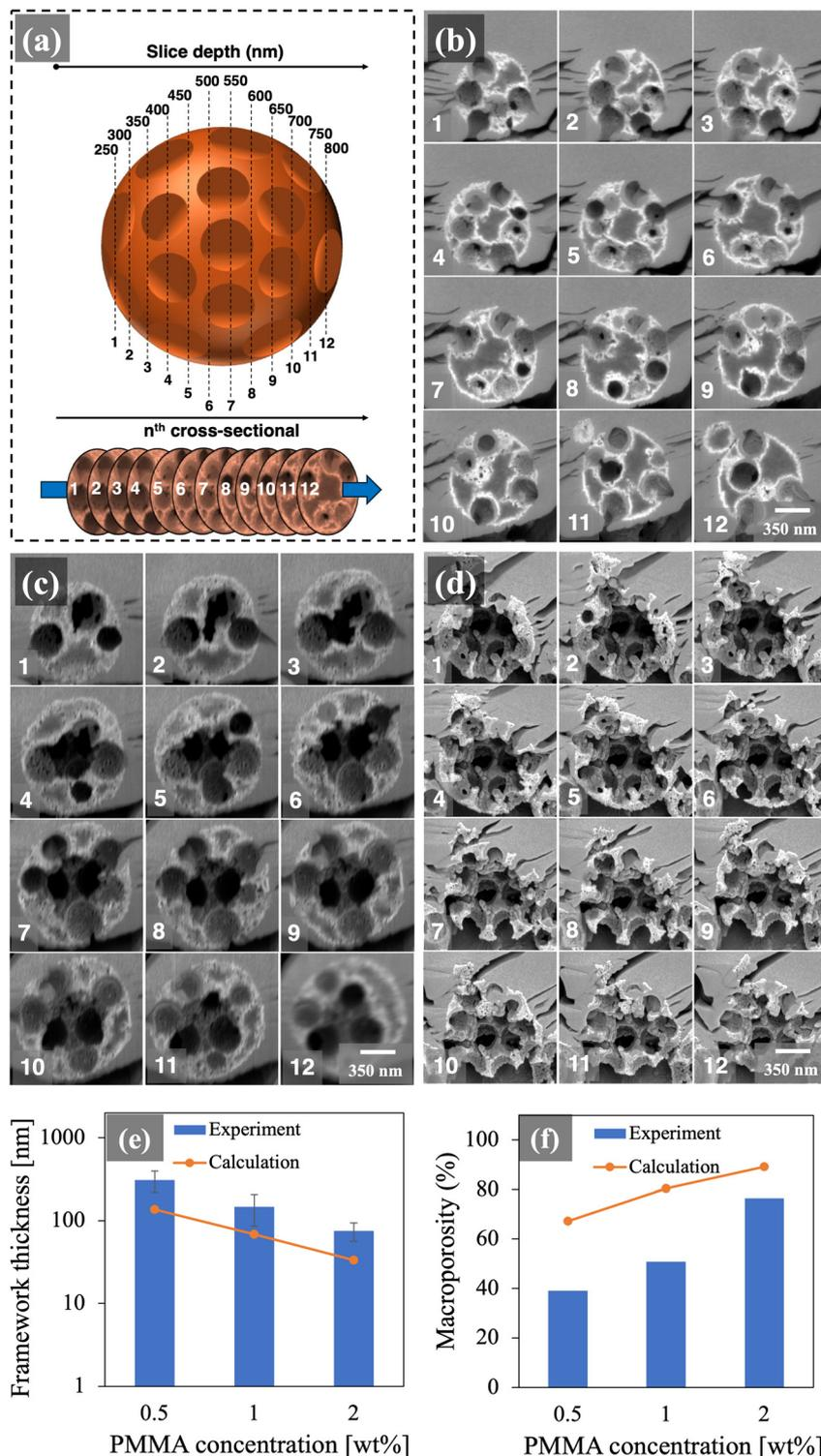
**Fig. 4** (a) Schematic illustration of the cutting plane for cross-sectional observations. FIB cross-sectional SEM images of porous TWC particles prepared at PMMA concentrations of (b) 0.5, (c) 1, and (d) 2 wt% and their (e) framework thicknesses and (f) macroporosities.
