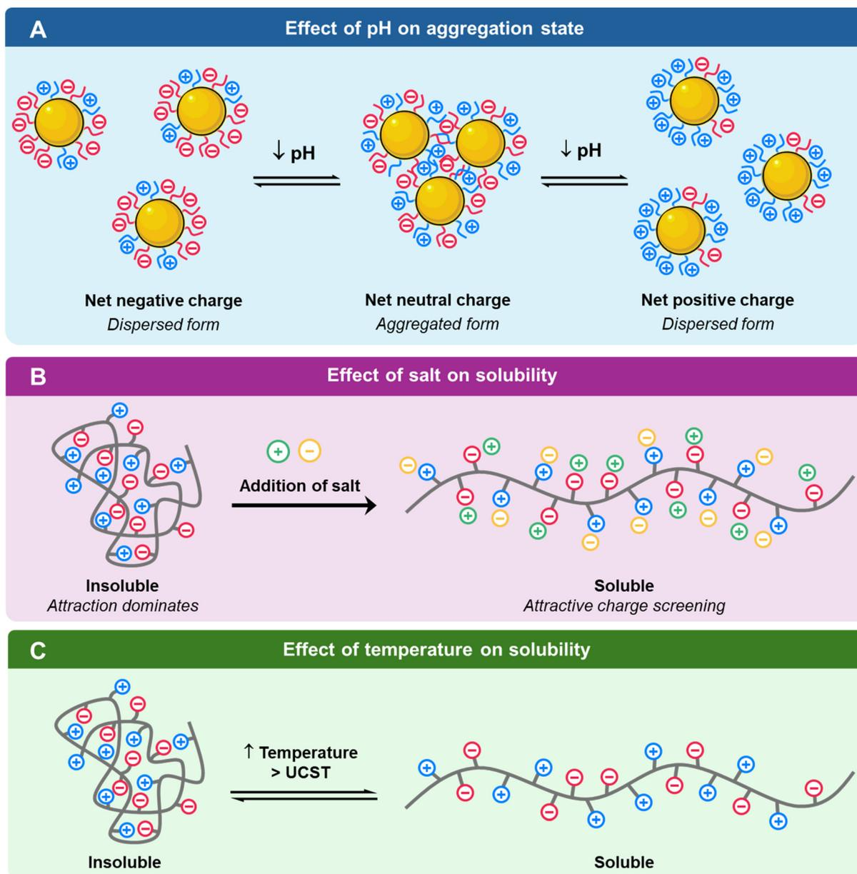
Fig. 3 Schematic of (A) pH, (B) salt addition and (C) temperature on the physical properties of charged nanomaterials.
