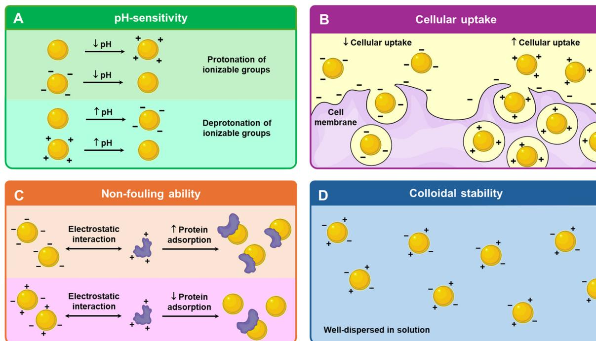
**Fig. 1** Benefits of charged nanomaterials. (A) Schematic of pH-sensitivity of charged nanoparticles. (B) Schematic of cellular uptake of negatively charged and positively charged nanoparticles. (C) Schematic of protein adsorption of negatively charged and mixed-charge nanoparticles. (D) Schematic of well-dispersed mixed charge nanoparticles in solution.
