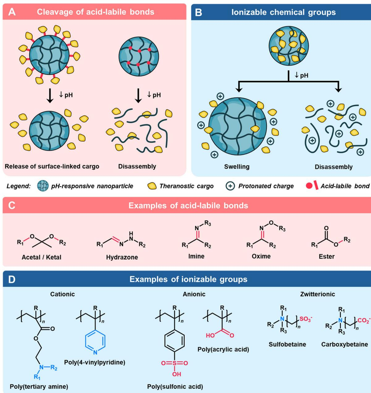
**Fig. 2** Overview of nanomaterial-based theranostic cargo delivery strategies using pH-triggered acid-labile bond cleavage and charge conversion. Schematic of (A) the mechanism of cargo release via cleavage of acid-labile bonds and (C) examples of such chemical bonds. A schematic of (B) the mechanism of cargo release via ionization of chemical groups and (D) examples of such groups.
