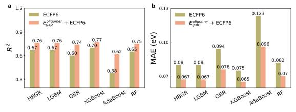
Fig. 4 (a) R<sup>2</sup> and (b) mean absolute error (MAE) (eV) of six machine learning models for predicting experimental optical gaps of conjugated polymers with different descriptors as input.  $E_{\text{qap}}^{\text{oligomer}}$  is HOMO-LUMO gap calculated from modified oligomer structures.
