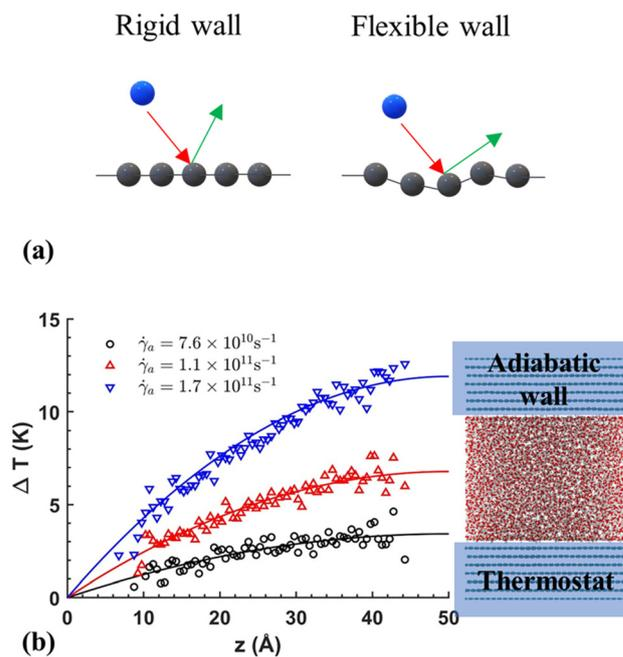
Fig. 7 (a) Schematic of rigid and flexible walls interacting with liquid particles in NEMD models, (b) temperature profile obtained by Shuvo *et al.*<sup>129</sup> (this figure has been adapted from ref. 129 with permission from AIP publishing, copyright 2024).
