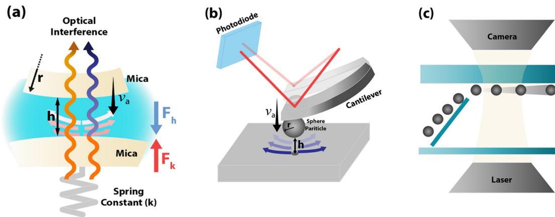
**Fig. 2** Schematic of the operational principles of (a) SFA, (b) AFM, and (c)  $\mu$ -PIV. In (a) and (b), the radius of the spherical probe ( $r$ ), surface separation distance ( $h$ ), and probe approach velocity ( $v_a$ ) are indicated as the parameters of the hydrodynamic drag force ( $F_h$ ) and the restorative force of the cantilever ( $F_k$ ), which are balanced for the hydrodynamic slip measurement.
