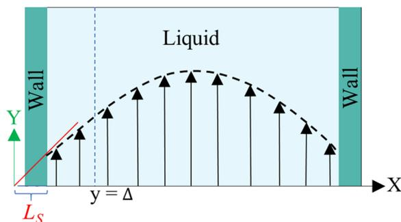
Fig. 9 Sketch of the system used in the friction analysis in Hansen *et al.*<sup>125</sup> This figure has been redrawn from ref. 125 with permission from American Physical Society, copyright 2011.
