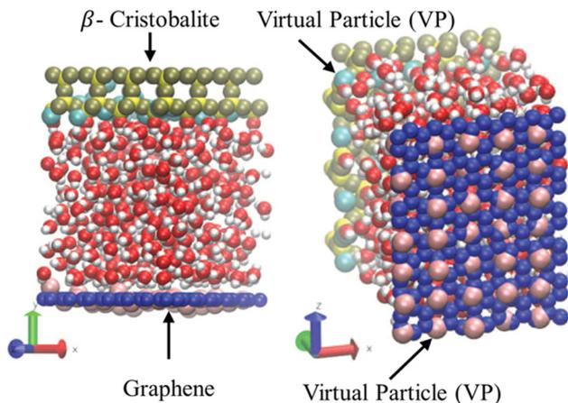
**Fig. 8** Computational domain of water confined between graphene sheets (dark blue spheres) and  $\beta$ -cristobalite (yellow spheres) wall with virtual particles (pink and light blue spheres). This figure has been adapted from ref. 133 with permission from American Chemical Society, copyright 2014.
