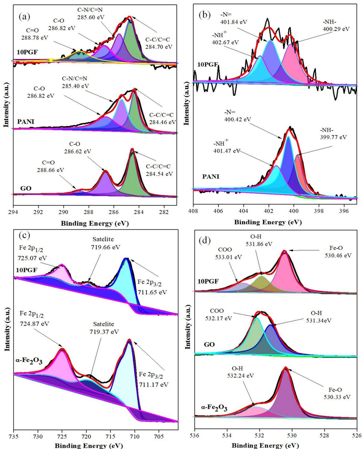
Fig. 5 High-resolution XPS spectra of pure PANI, GO, and  $\alpha$ -Fe<sub>2</sub>O<sub>3</sub> and the 10PGF ternary composite for C 1s (a), N 1s (b), Fe 2p (c), and O 1s (d).
