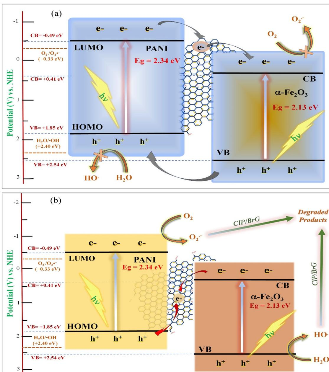
Fig. 10 Conventional mechanism (a) and Z-scheme mechanism (b) for the 10PGF heterostructure.
