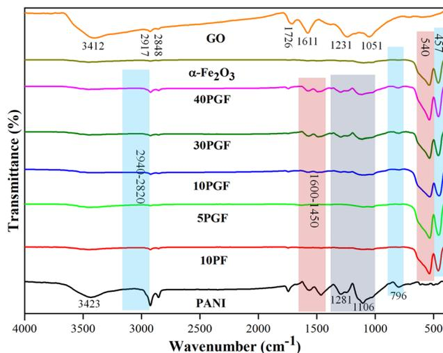
Fig. 2 FTIR spectra of pure GO, PANI, and  $\alpha$ -Fe<sub>2</sub>O<sub>3</sub>, the 10PF binary composite and various PGF ternary composites.
