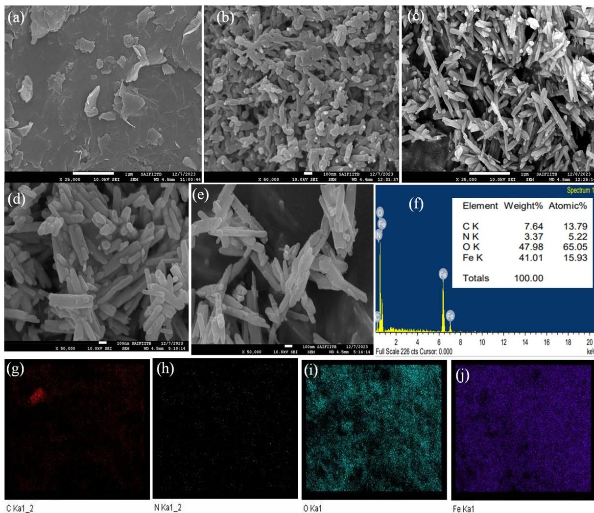
**Fig. 3** FE-SEM images of GO (a), PANI (b),  $\alpha\text{-Fe}_2\text{O}_3$  (c), and the 10PGF ternary composite (d and e). EDX spectra with at% and wt% values of the elements (f) and elemental mapping of the 10PGF ternary composite (g–j).
