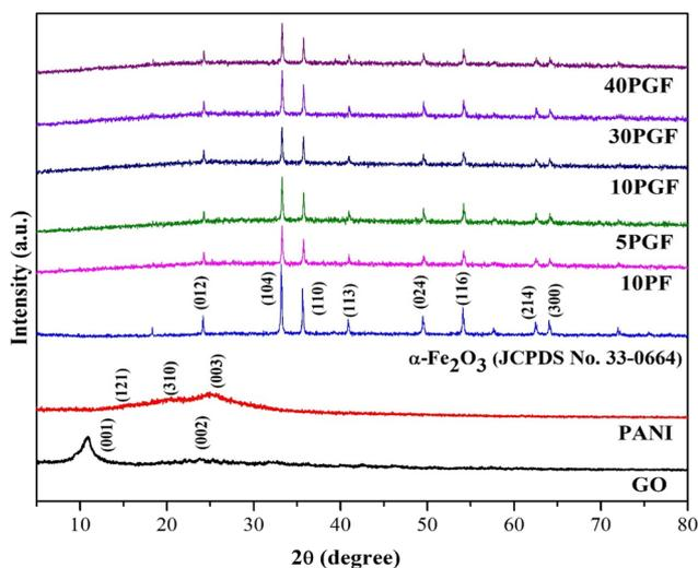
Fig. 1 XRD patterns of pure GO, PANI, and  $\alpha$ -Fe<sub>2</sub>O<sub>3</sub>, the 10PF binary composite and the PGF ternary composites.
