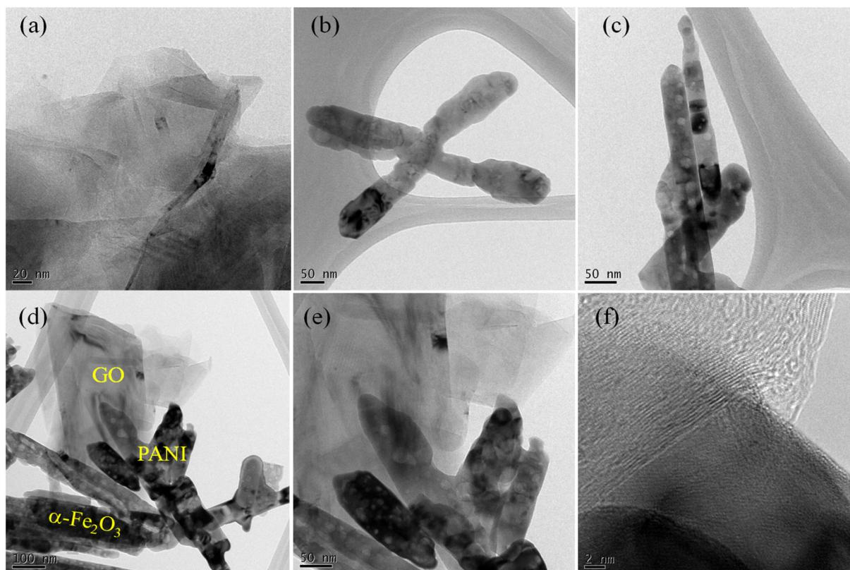
Fig. 4 TEM images of GO (a), PANI (b),  $\alpha$ -Fe<sub>2</sub>O<sub>3</sub> (c) and 10PGF (d–f).
