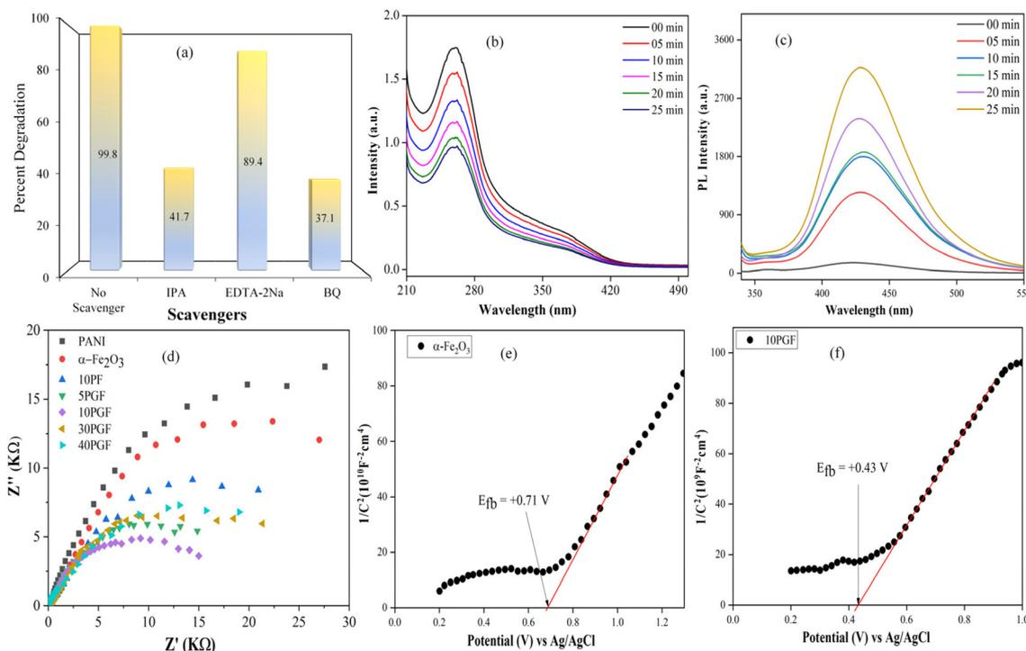
**Fig. 9** Trapping experiment results (a), decrease in NBT spectra (b) and increase in the PL intensity of TA-OH (c) with the 10PGF composite. EIS Nyquist plots of all the photocatalysts (d); Mott–Schottky plots for  $\alpha$ -Fe<sub>2</sub>O<sub>3</sub> (e) and the 10PGF composite (f).
