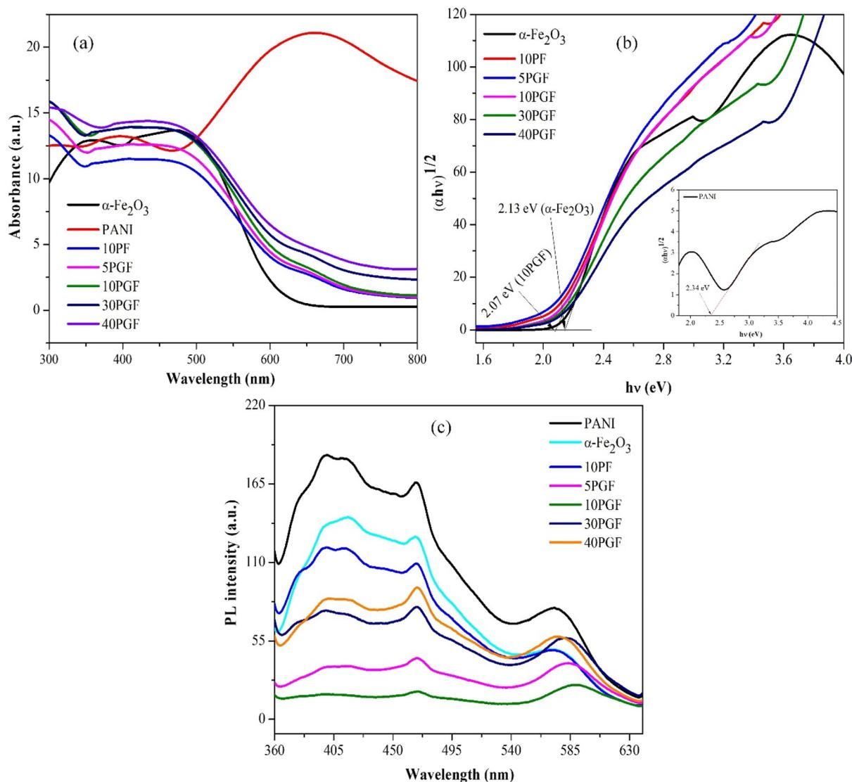
**Fig. 7** UV–vis DRS spectra of pure  $\alpha$ -Fe<sub>2</sub>O<sub>3</sub>, pure PANI, the 10PF binary composite and various ternary composites (a), the respective Tauc plots (b) and PL spectra of the photocatalysts (c).
