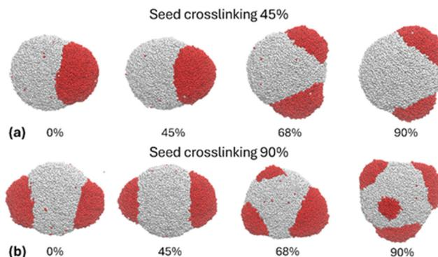
**Fig. 10** The DPD simulations showing the effect of polymer chain entanglements between the seed (white beads) and second polymer (red beads) networks on the distinct final morphologies of JPs for cross-linking degrees of 0%, 45%, 68%, and 90% for the second polymer. Panels (a) and (b) compare the 45% and 90% crosslinked seeds, respectively. Reproduced from ref. 124 with permission from Elsevier. Copyright 2019.
