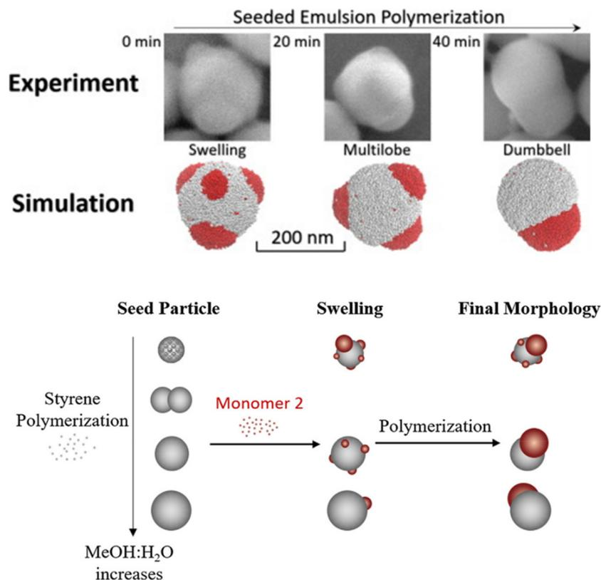
**Fig. 9** Schematic illustration of morphology evolution during the seeded emulsion polymerization. The morphologies are significantly impacted by the crosslinking density and solvent choice during seed synthesis. The morphology can be controlled through polymerization kinetics. Reproduced from ref. 124 with permission from Elsevier. Copyright 2019.
