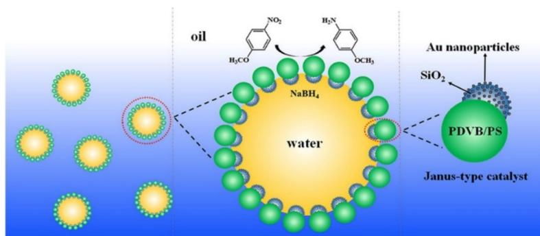
**Fig. 14** Schematic illustration of how the Janus-type catalyst can stabilize a water-in-oil emulsion and exhibit high catalytic activity for the reduction of nitro-compounds at the emulsion interface. Reproduced from ref. 14 with permission from Elsevier. Copyright 2017.
