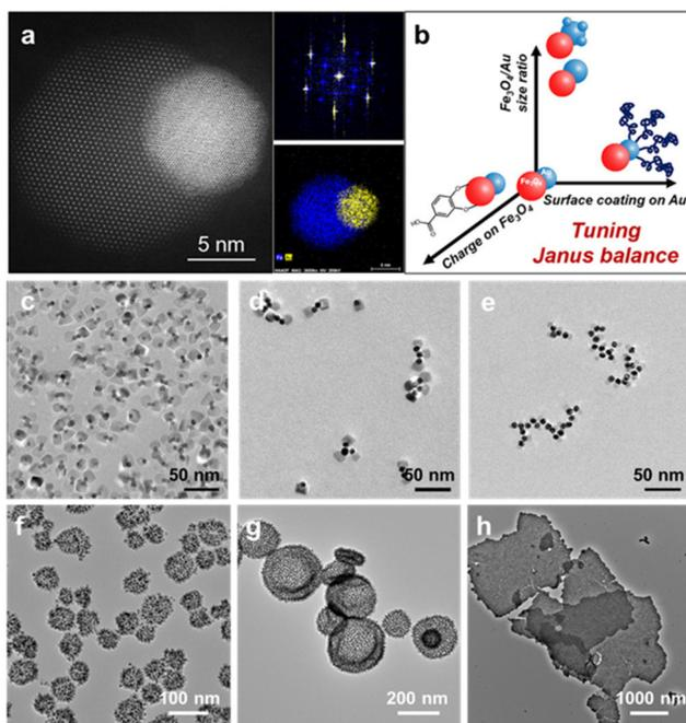
**Fig. 2** (a) HAADF-STEM image of a typical Au-Fe<sub>3</sub>O<sub>4</sub> nanocrystal and its corresponding fast FFT patterns and EDS elemental mapping. (b) Strategies for tuning of the Janus balance of Au-Fe<sub>3</sub>O<sub>4</sub> nanocrystals. (c–h) Self-assembly structures of Au-Fe<sub>3</sub>O<sub>4</sub> nanocrystals, including clusters, chains, micelles, capsules, and sheets. Reproduced from ref. 95 with permission from the American Chemical Society. Copyright 2019.
