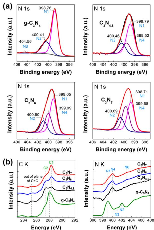
Fig. 4 (a) N 1s XPS spectra and (b) (left) C K- and (right) N K-edge NEXAFS spectra of exfoliated  $g\text{-C}_3\text{N}_4$ ,  $\text{C}_3\text{N}_{4.8}$ ,  $\text{C}_3\text{N}_6$ , and  $\text{C}_3\text{N}_7$  nanosheets.
