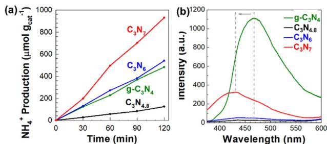
Fig. 6 (a) Amount of generated ammonia under a N<sub>2</sub> atmosphere and (b) PL spectra for exfoliated g-C<sub>3</sub>N<sub>4</sub>, C<sub>3</sub>N<sub>4.8</sub>, C<sub>3</sub>N<sub>6</sub> and C<sub>3</sub>N<sub>7</sub> nanosheets.
