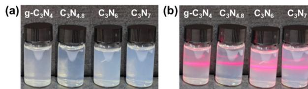
**Fig. 2** (a) Photographs and (b) Tyndall phenomenon of colloidal suspensions of exfoliated  $g-C_3N_4$ ,  $C_3N_{4.8}$ ,  $C_3N_6$ , and  $C_3N_7$  nanosheets.
