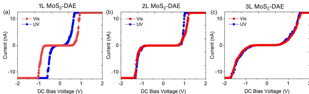
**Fig. 3** Conductive AFM measurements on photoswitched hybrid samples under UV and visible irradiation: (a) 1L MoS<sub>2</sub>-DAE, (b) 2L MoS<sub>2</sub>-DAE, and (c) 3L MoS<sub>2</sub>-DAE. Bias DC voltage was applied from  $-2$  V to  $2$  V and currents were recorded within  $\pm 12$  nA. UV light enhances the current significantly in 1L MoS<sub>2</sub>-DAE, whereas no significant changes are observed from the hybrids with 2L and 3L MoS<sub>2</sub>.
