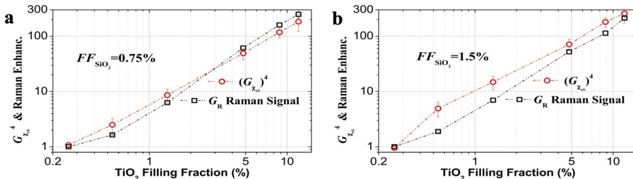
Fig. 4 Comparison of the Raman enhancement measured using a glass slide to cover the samples,  $G_R$  (black open squares), and fourth power of the electric susceptibility enhancement,  $(G_{xe})^4$  (red open circles), for the samples with (a)  $FF_{SiO_2} = 0.75\%$  and (b)  $FF_{SiO_2} = 1.5\%$ .
