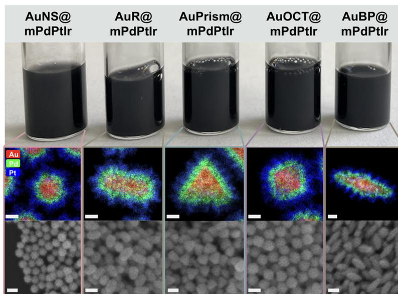
**Fig. 2** Photographs of the nanoparticle solutions, TEM-EDS elemental maps and SEM images of the multimetallic nanoparticles containing a gold core with spherical, rod-shaped, prism-shaped, octahedral, and bipyramidal morphology (left to right). The spatial distribution of the elements is color coded. Scale bars are 20 nm and 100 nm for TEM and SEM images, respectively.
