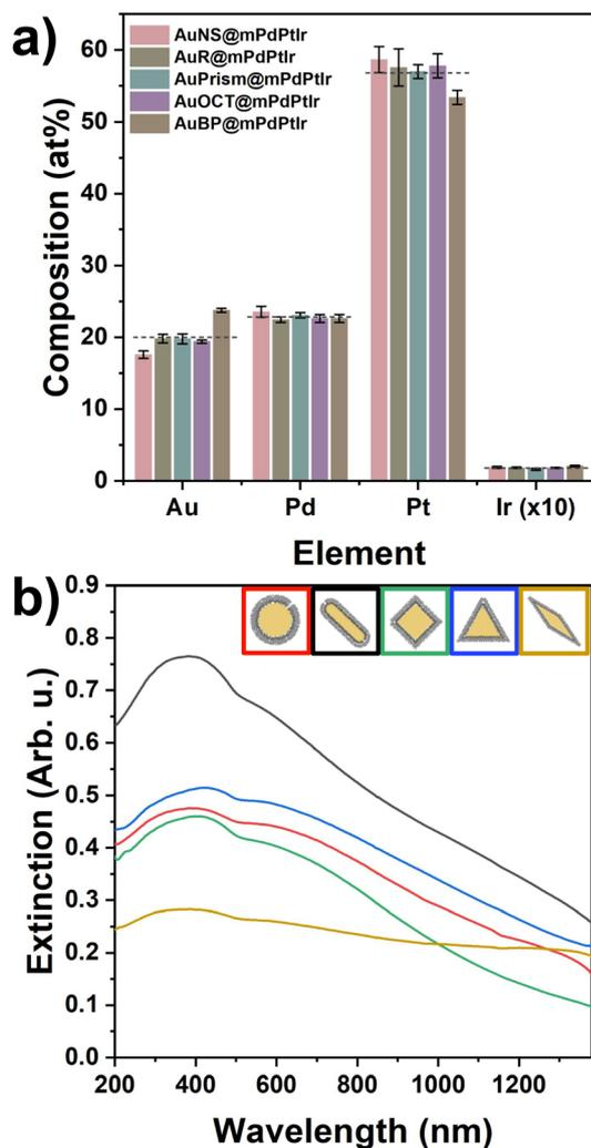
**Fig. 3** Elemental composition (in atomic%) of the different tetrametallic nanoparticles measured by ICP-OES (a). Dashed lines represent the mean value of the corresponding elements in the five different nanoparticle model systems. UV-Vis-NIR extinction spectra of the tetrametallic nanoparticles (b).
