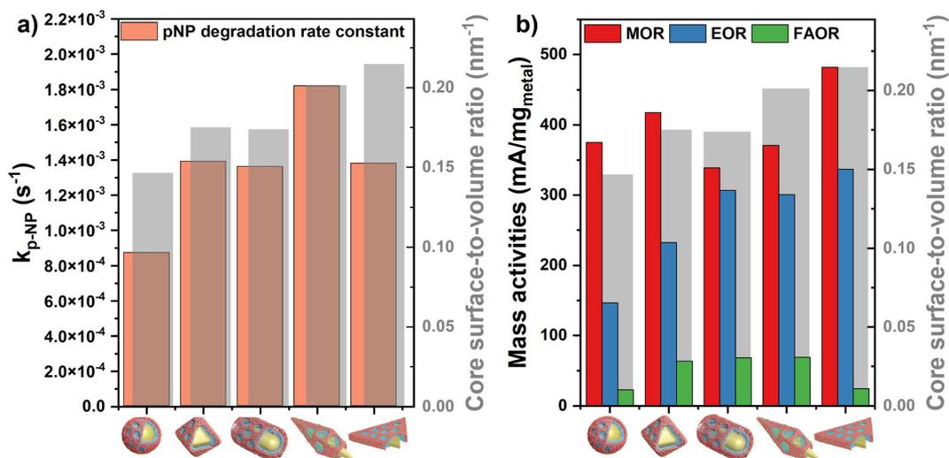
**Fig. 8** Comparison of the catalytic performance of the tetrametallic nanoparticles with different core morphologies in the degradation reaction of *p*-nitrophenol (a) and electrooxidation reactions (b). Gray bars represent the surface-to-volume ratios of the corresponding Au core particles.
