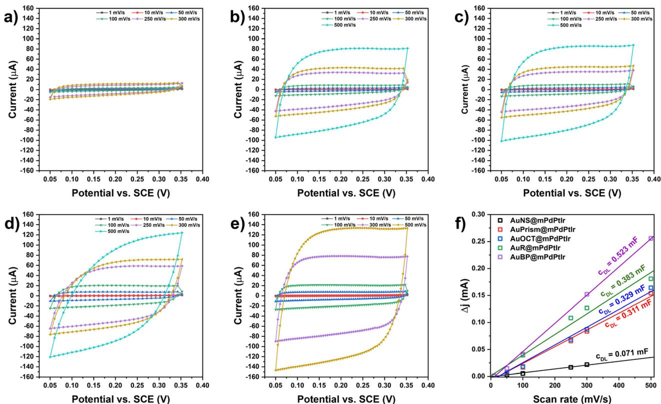
**Fig. 6** Scan rate dependent CV curves of GCE electrodes modified by multimetallic nanoparticles with spherical (a), prism-shaped (b), octahedral (c), rod-shaped (d), and bipyramidal (e) cores in 1 M KOH electrolyte. Double layer capacitances for the different types of multimetallic nanoparticle electrodes (f).
