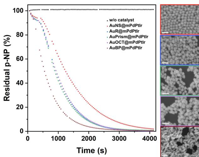
Fig. 5 Residual *p*-nitrophenol in % as a function of time for the investigated model systems calculated from the measured absorbance at 400 nm over time. All decay curves represent the average of at least three consecutive measurements. Insets show the SEM images of the particles (color coded to the absorbance data) collected after the catalytic reaction by centrifugation (scale bars are 200 nm).
