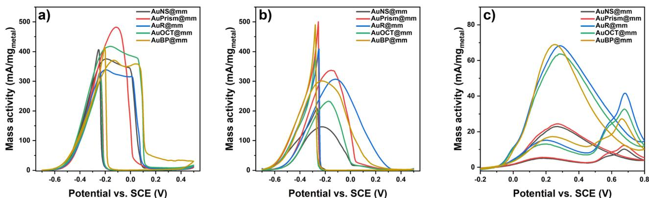
**Fig. 7** Mass activity of different types of multimetallic nanoparticle electrodes in the MOR (a), EOR (b) and FAOR (c). The total metal concentration was kept constant during the preparation of all electrodes.
