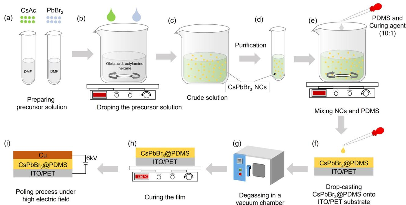
**Fig. 1** Schematic illustration outlining the entire fabrication process of PNG devices. (a–d) Synthesis process of CsPbBr<sub>3</sub> NCs. (e–h) Fabrication process of the CsPbBr<sub>3</sub>@PDMS composite film. (i) Assembly and polarization of PNG devices.
