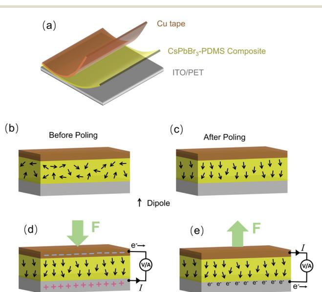
**Fig. 3** (a) Schematic diagram of the  $\text{CsPbBr}_3$  NCs@PDMS composite PNG. The arrangement of electric dipoles in  $\text{CsPbBr}_3$  NCs (b) before and (c) after high voltage polarization of the PNG device. Power generation under (d) pressing and (e) releasing modes of the PNG device.
