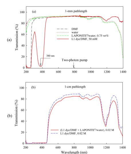
Fig. 2 Transmission spectra of (a) four 1 mm solution samples and (b) two 1 cm solution samples.
