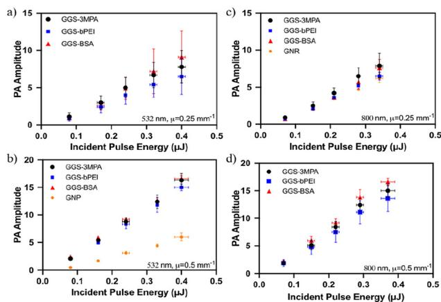
Fig. 5 Photoacoustic spectroscopy results of GGS samples having (a and c) 0.25  $\text{mm}^{-1}$  and (b and d) 0.5  $\text{mm}^{-1}$  extinction coefficients at 532 and 800 nm, respectively. Data were shown as mean  $\pm$  SD ( $n = 3$ ).
