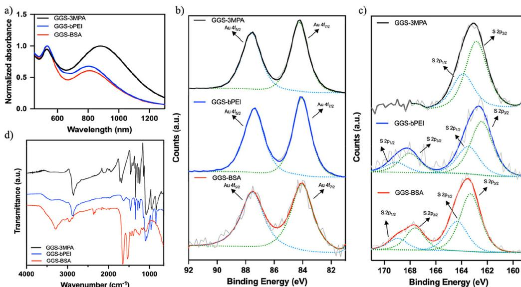
**Fig. 1** (a) The UV–VIS spectra, (b) Au 4f and (c) S 2p XPS spectra, (d) FTIR spectra of the GGS-3MPA, GGS-bPEI, and GGS-BSA.
