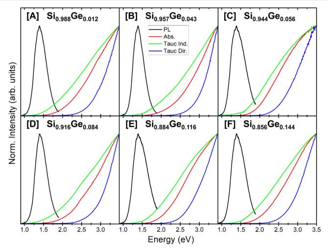
Fig. 5 Solid-state PL (black), Kubelka-Munk converted absorption (red), direct (blue) and indirect (green) Tauc spectra of [A] Si<sub>0.988</sub>Ge<sub>0.012</sub>, [B]  $Si_{0.957}Ge_{0.043}$ , [C]  $Si_{0.944}Ge_{0.056}$ , [D]  $Si_{0.916}Ge_{0.084}$ , [E]  $Si_{0.884}Ge_{0.116}$ , and [F]  $Si_{0.856}Ge_{0.144}$  alloy NCs.
