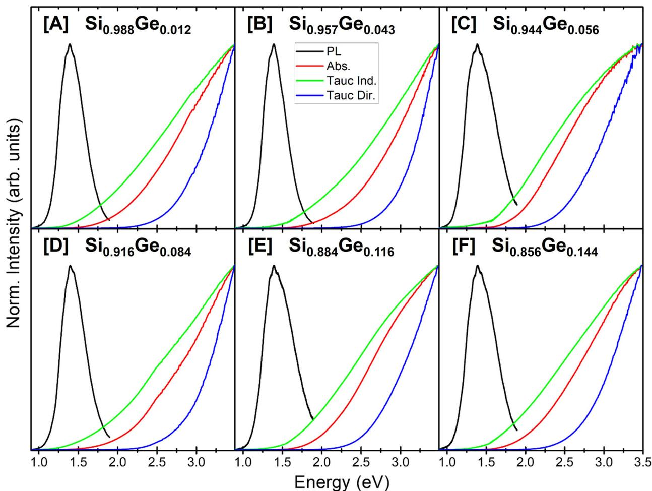
Fig. 5 Solid-state PL (black), Kubelka–Munk converted absorption (red), direct (blue) and indirect (green) Tauc spectra of [A]  $\text{Si}_{0.988}\text{Ge}_{0.012}$ , [B]  $\text{Si}_{0.957}\text{Ge}_{0.043}$ , [C]  $\text{Si}_{0.944}\text{Ge}_{0.056}$ , [D]  $\text{Si}_{0.916}\text{Ge}_{0.084}$ , [E]  $\text{Si}_{0.884}\text{Ge}_{0.116}$ , and [F]  $\text{Si}_{0.856}\text{Ge}_{0.144}$  alloy NCs.
