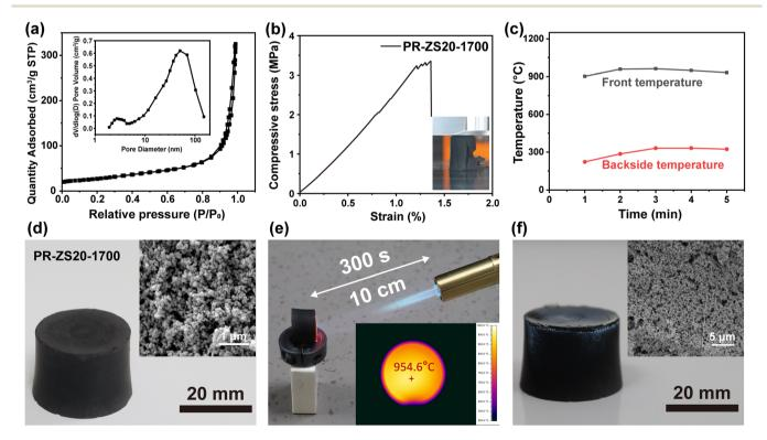
Fig. 8 (a) N<sub>2</sub> adsorption – desorption isotherms and BJH pore size distribution curve, (b) compressive stress – strain curve, and (c) front and backside temperatures during the ablation of PR-ZS20-1700. (d) Pristine sample, (e) sample during burning test, and (f) sample after burning test.
