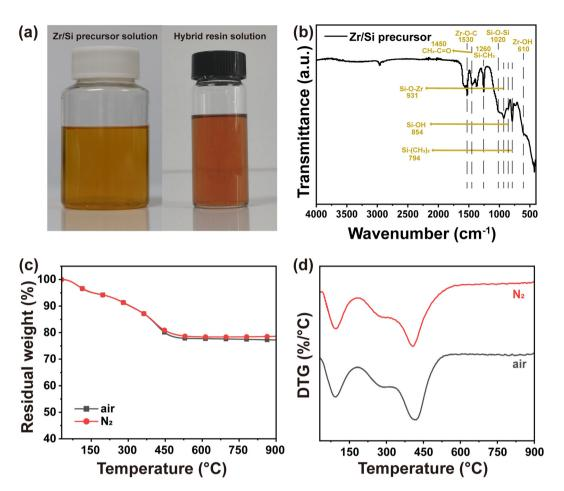
Fig. 2 (a) Digital photos of Zr/Si precursor solution and hybrid resin solution, (b) FTIR spectrum, (c) TGA and (d) DTG curves in air and N<sub>2</sub> atmosphere of Zr/Si precursor.
