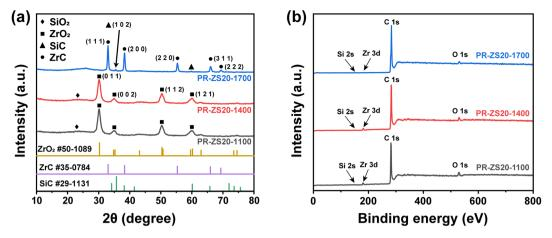
Fig. 7 (a) XRD patterns and (b) XPS spectra of PR-ZS20-1100, PR-ZS20-1400, and PR-ZS20-1700.
