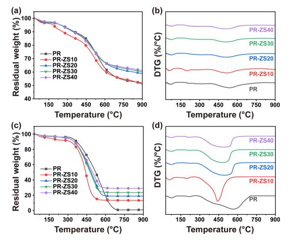
Fig. 4 TGA and DTG curves of PR and PR-ZS aerogels in (a and b) N<sub>2</sub> and (c and d) air atmospheres.
