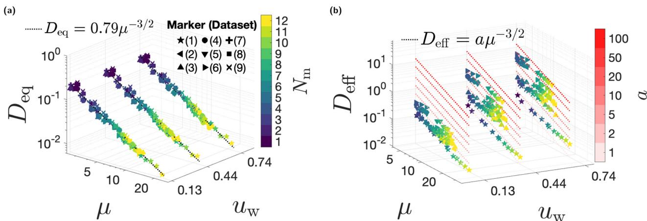
**Fig. 3** Viscosity and wall velocity dependence of (a) the spanwise coefficient of self-diffusion and (b) the streamwise coefficient of self-diffusion. In both cases, models of the viscosity-dependent form discussed in Sukhishvili *et al.*<sup>30</sup> are overlaid. Contours of constant pre-factor  $a$  are provided as a guide to the eye in (b).
