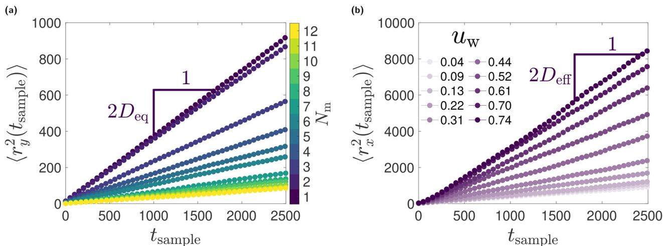
**Fig. 2** (a) Characteristic MSDs in the spanwise direction (drawn from dataset 4 and averaged over all wall velocities) as a function of sampling time and polymer chain length, which are used to measure  $D_{\text{eq}}$ ; (b) characteristic MSDs in the streamwise direction for a monomeric fluid ( $N_m = 1$ ) as a function of sampling time and wall velocity, which are used to measure  $D_{\text{eff}}$ .
