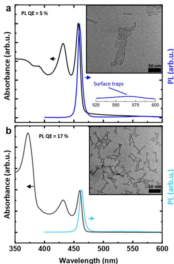
**Fig. 1** (a) Normalized absorbance (black) and photoluminescence (blue) spectra, and TEM image of initial (before DoE optimization) 3.5 ML CdSe NPLs. In the spectral region of 525–600 nm, a broadband emission is observed, arising from surface traps. (b) Normalized absorbance (black) and photoluminescence (blue) spectra, and TEM image of the 3.5 ML CdSe NPLs after growth of a CdS crown.
