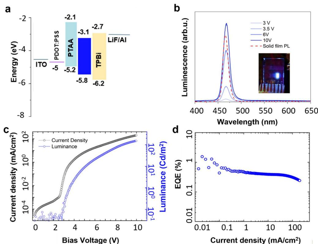
**Fig. 6** (a) Energy band diagram of the LED structure. (b) Electroluminescence spectra under different bias voltages (blue), and photoluminescence of a comparable solid film (red) (c) current density and luminance of a typical LED plotted against applied bias. (d) External quantum efficiency of a typical LED plotted against current density.
