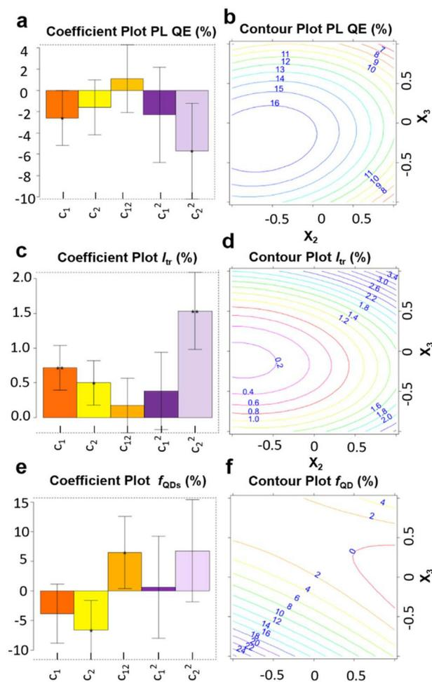
**Fig. 3** Coefficients plot and contour plots for the three responses of CCF design (PL QE (a, b),  $I_{tr}$  (c, d) and  $f_{QD}$  (e, f)). Black bars in the coefficient plots (a, c, e) represent confidence intervals of each coefficient. Contour plots (b, d, f) are constructed using the two input factors  $X_2$  (cadmium stearate amount),  $X_3$  (propionic acid amount).
