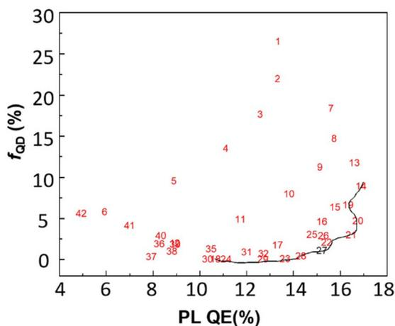
**Fig. 4** Experimental conditions (red) found through a Pareto front algorithm of PL QE and  $f_{\text{QD}}$ . The Pareto front (black line) is represented by non-dominated points. Experiment 27 (black) has been selected as the optimal solution.
