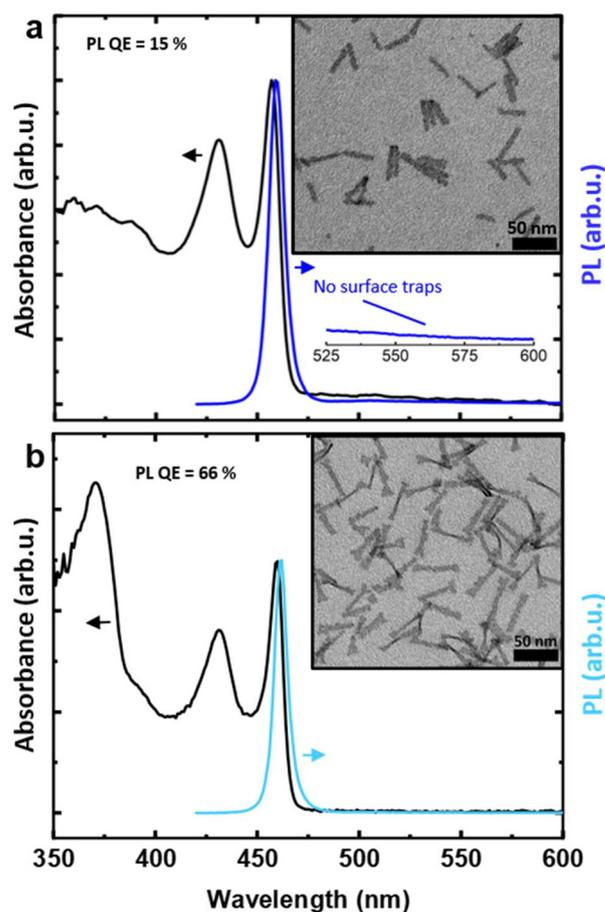
**Fig. 5** (a) Normalized absorbance (black) and photoluminescence (blue) spectra, and TEM image of final (after DoE optimization) 3.5 ML CdSe NPLs. In the spectral region of 525–600 nm, no broadband emission, arising from surface traps, is observed. (b) Normalized absorbance (black) and photoluminescence (blue) spectra, and TEM image of the same 3.5 ML, after growth of a CdS crown.
