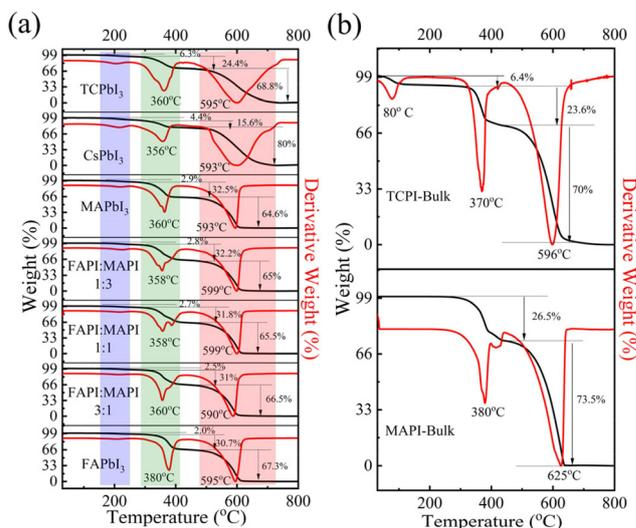
**Fig. 5** TG curves and their corresponding DTG plots of (a)  $\text{TCPbI}_3$ ,  $\text{CsPbI}_3$ ,  $\text{FAPbI}_3$ ,  $\text{MAPbI}_3$  and  $\text{FA}_x\text{MA}_{1-x}\text{PbI}_3$  PNCs, and (b) the  $\text{MAPbI}_3$  and  $\text{TCPbI}_3$  bulk thin-film perovskites. The percentage mass loss in the three different steps is shown by the arrow along with the corresponding value.
