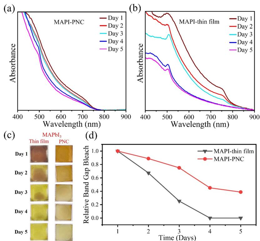
**Fig. 2** UV-vis absorption spectra of (a) the MAPI PNC film and (b) the MAPI thin film recorded from day 1 to day 5 after preparation in 50–70% relative humidity (RH) under normal light and ambient conditions. (c) Photographs of both the MAPI PNC and thin films showing how the colour of the film changes with time. (d) Comparison of the change of relative absorption of both films with time; the PNC film shows better phase stability compared with the thin film.
