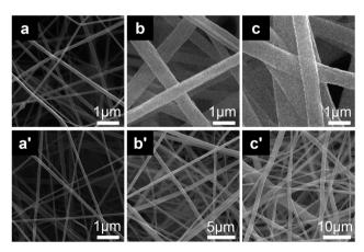
**Fig. 3** SEM photographs of QFD-doped PVC fiber films at different precursor concentrations and voltages in electrostatic spinning. (a, a') 10 wt%, 15 kV; (b, b') 15 wt%, 15 kV; and (c, c') 15 wt%, 10 kV.
