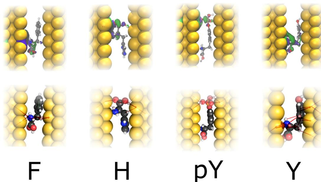
**Fig. 4** Top row: WF corresponding to an energy of  $E - E_F = 0.0$  eV; bottom row: respective LC for Phe(F), His(H) Tyr modified (pY) and Tyr (Y) in the infinite capacitor device (7.0 Å between the gold layers). Atomic color: yellow (Au), gray (C), red (O), blue (N), orange (P) and white (H); purple spheroids (positive WF portion); green spheroids (negative WF portion).
