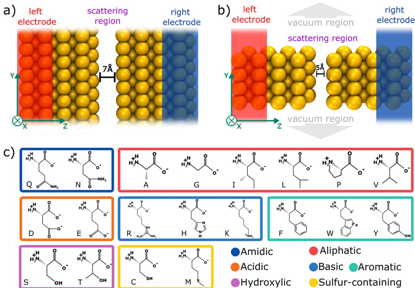
**Fig. 1** (a) Schematic of an infinite capacitor schematic with a 7.0 Å spacing in an electronic device; (b) 5.0 Å nanojunction; insets provide an atomic-level view of the structure; (c) chemical structure of amino acids, followed by their 1-letter codes and organized based on their main characteristics.
