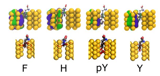
Fig. 5 Top row: WF corresponding to an energy of  $E - E_F = 0$  eV; bottom row: respective local currents (LC) for Phe(F), His(H), Tyr modified (pY), and Tyr (Y) amino in the tip 5.0 Å. Atomic color: yellow (Au), gray (C), red (O), blue (N), orange (P) and white (H); purple spheroids (positive WF portion); green spheroids(negative WF portion). 5 Å nanojunction device.
