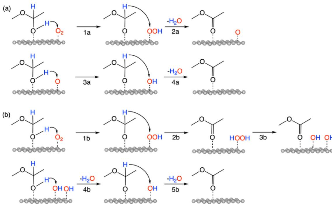
**Scheme 2** Oxidative dehydrogenation of a hemiacetal: (a) the \_oxo pathway; (b) the \_H<sub>2</sub>O<sub>2</sub> pathway.
