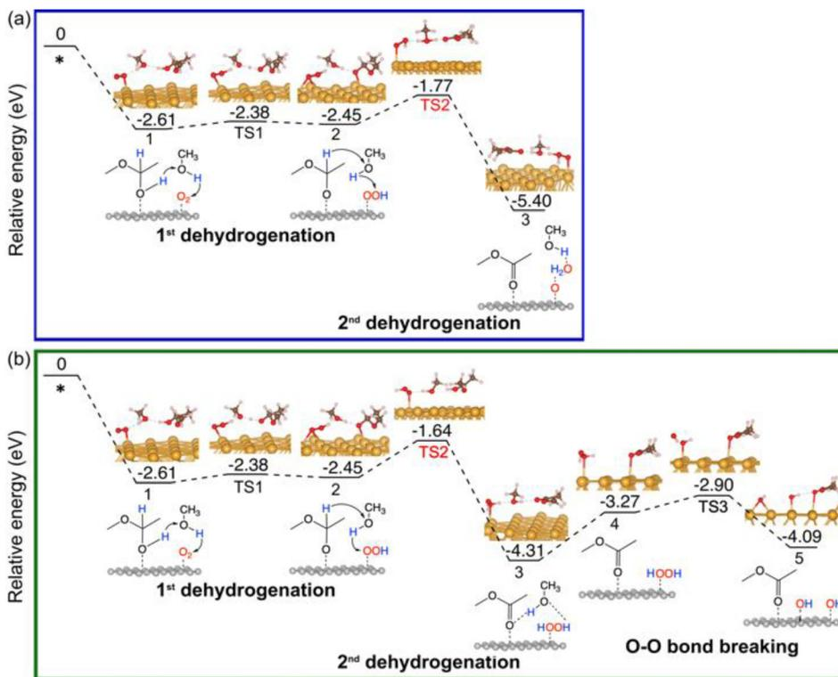
Fig. 5 Energy profiles of the oxidative dehydrogenation of the 1<sup>st</sup> hemiacetal on Au (111): (a) via the  $\text{O}_2$  pathway; (b) via the  $\text{H}_2\text{O}_2$  pathway.
