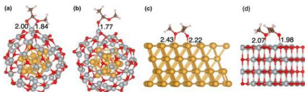
**Fig. 7** Adsorption structures and modes of a deprotonated hemiacetal: (a) bidentate on Au<sub>13</sub>@(NiO)<sub>48</sub>; (c) monodentate on Au<sub>13</sub>@(NiO)<sub>48</sub>; (c) bridging on Au(111); and (d) bridging on NiO(100). Ni–O and Au–O distances are given in Å.
