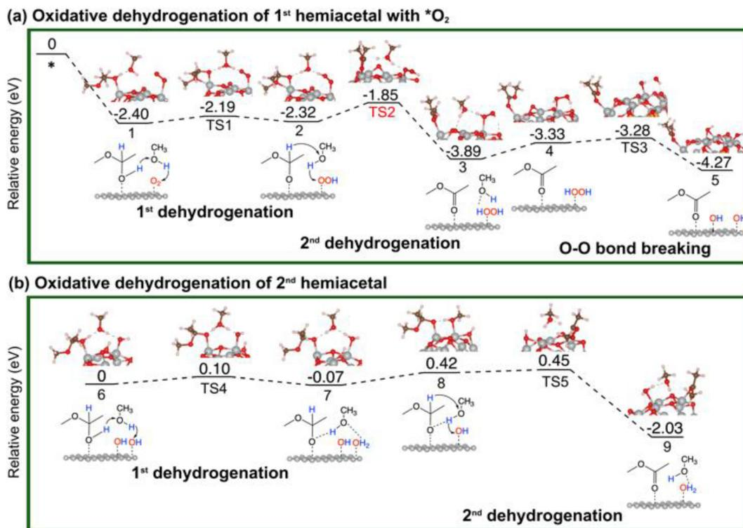
Fig. 4 Energy profiles and key structures of the oxidative dehydrogenation of a hemiacetal to produce ester and water molecules *via* the  $\text{H}_2\text{O}_2$  pathway on  $\text{Au}_{13}@\text{NiO}_{48}$ : (a) formation of the 1<sup>st</sup> ester; (b) formation of the 2<sup>nd</sup> ester.
