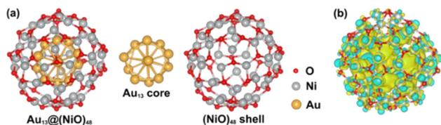
**Fig. 1** (a) Structures of the Au<sub>13</sub>@(NiO)<sub>48</sub> core-shell model, the Au<sub>13</sub> core, and the (NiO)<sub>48</sub> shell. (b) Charge density difference plot (isosurface values are  $\pm 6.6 \times 10^{-4} \text{ e } \text{\AA}^{-3}$ ): yellow, electron accumulation; cyan, electron depletion. Note that the Au<sub>13</sub> core geometry in (a) slightly deforms from the perfect icosahedral shape due to the interaction with the shell.
