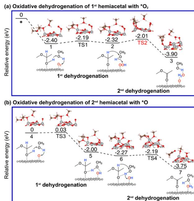
**Fig. 3** Energy profiles and key structures of the oxidative dehydrogenation of a hemiacetal to produce ester and water molecules *via* the *\_oxo* pathway on Au<sub>13</sub>@(NiO)<sub>48</sub>: (a) formation of the 1<sup>st</sup> ester; (b) formation of the 2<sup>nd</sup> ester.
