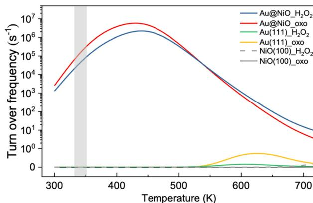
**Fig. 8** Microkinetic modeling of the oxidative dehydrogenation of a hemiacetal to produce esters on Au<sub>13</sub>@(NiO)<sub>48</sub>, Au(111), and NiO(100) and water molecules via the *\_oxo* and *\_H<sub>2</sub>O<sub>2</sub>* pathways. The gray area indicates the experimental temperature range for this reaction.
