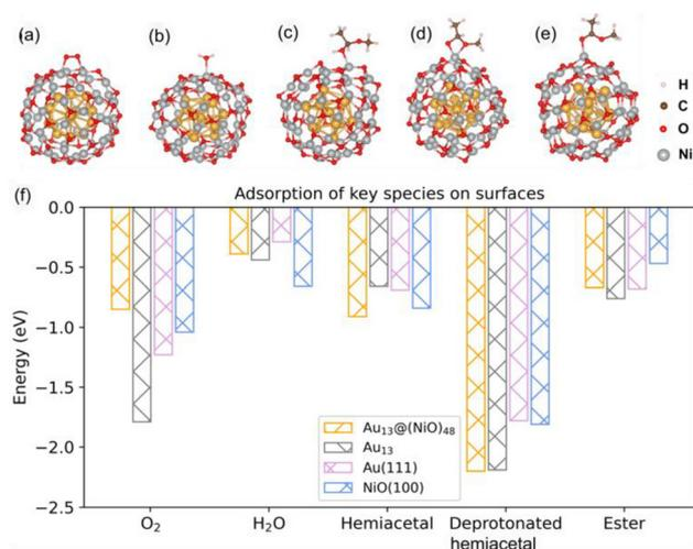
**Fig. 2** Optimized adsorption structures on the Au<sub>13</sub>@(NiO)<sub>48</sub> core-shell nanocatalyst: (a) O<sub>2</sub>; (b) H<sub>2</sub>O; (c) hemiacetal; (d) deprotonated hemiacetal; (e) ester; and (f) adsorption energies on Au<sub>13</sub>@(NiO)<sub>48</sub>, Au<sub>13</sub>, Au(111), and NiO(100).
