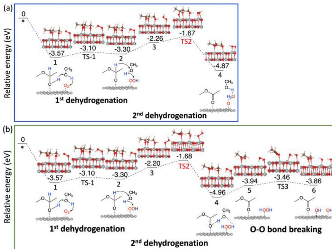
Fig. 6 Energy profiles of the oxidative dehydrogenation of the 1<sup>st</sup> hemiacetal on NiO(100): (a) via the  $\text{O}_2$  pathway; (b) via the  $\text{H}_2\text{O}_2$  pathway.
