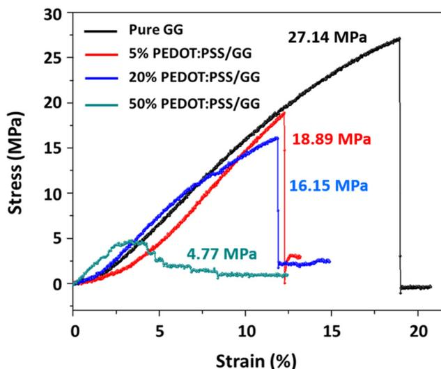
Fig. 9 Stress-strain curves of the PEDOT:PSS/GG composite membranes.
