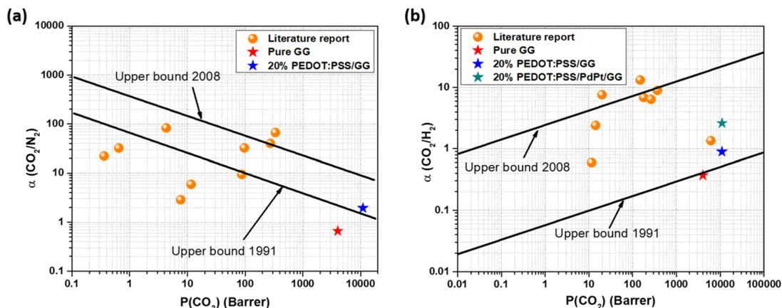
Fig. 11 Comparative assessment of gas separation performance against the Robeson upper bound and previously published work for (a)  $\text{CO}_2/\text{N}_2$  and (b)  $\text{CO}_2/\text{H}_2$  separation.
