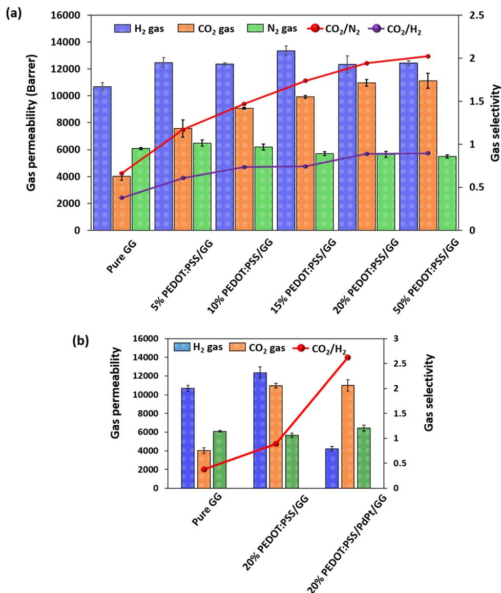
Fig. 10 Gas separation performances of the PEDOT:PSS/guar gum composite membranes at 10 psi pressure (a) at different wt% values of guar gum and (b) with bimetallic PdPt nanoparticles.
