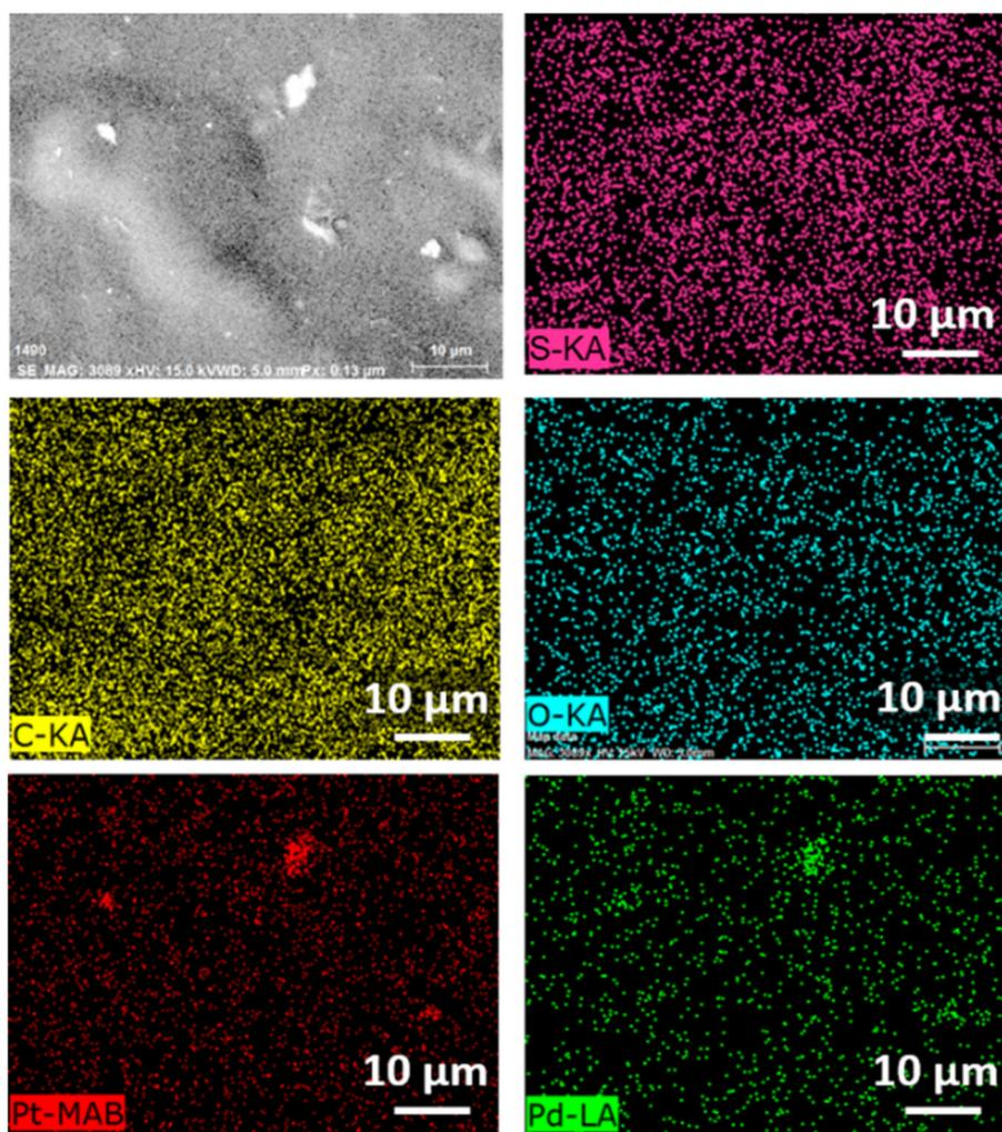
Fig. 8 Top-surface EDS mapping images of S, C, O, Pt, and Pd elements in the 20% PEDOT:PSS/PdPt/GG composite membranes.
