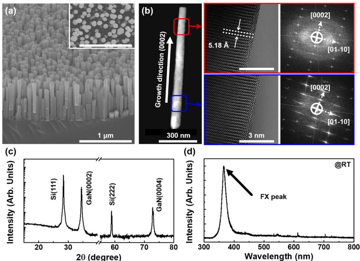
**Fig. 1** (a) Three-dimensional FE-SEM images of GaN NWs. Inset: plan-view image. (b) TEM (left) and HR-TEM (middle) image and SAED patterns (right) of a single GaN NW measured at two different vertical positions. (c) XRD rocking curve and (d) PL spectrum of GaN NWs.
