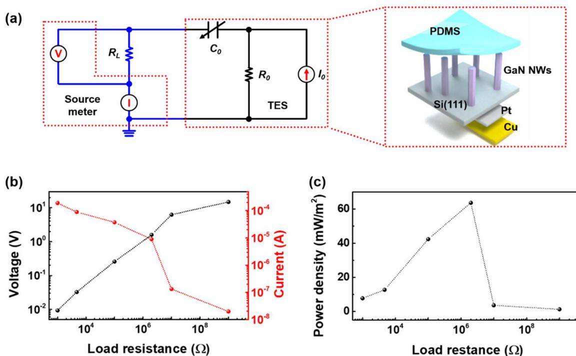
Fig. 4 (a) Simplified equivalent circuit model connected with a source meter and the layout of the TES. (b) Summary of average output voltage and current of the TES as a function of  $R_L$ . (c) Calculated power density of the TES as a function of  $R_L$ .
