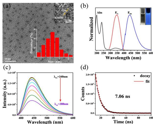
**Fig. 1** (a) TEM and HRTEM images of N-S-CDs (inset: histogram of particle size distribution); (b) normalized UV-vis and FL spectra of N-S-CDs (inset: corresponding photos under sunlight (left) and 365 nm ultraviolet light (right)); (c) PL spectra of N-S-CDs at different excitation wavelengths; and (d) time resolved decay spectra and fluorescence lifetime fitting curves of N-S-CDs.
