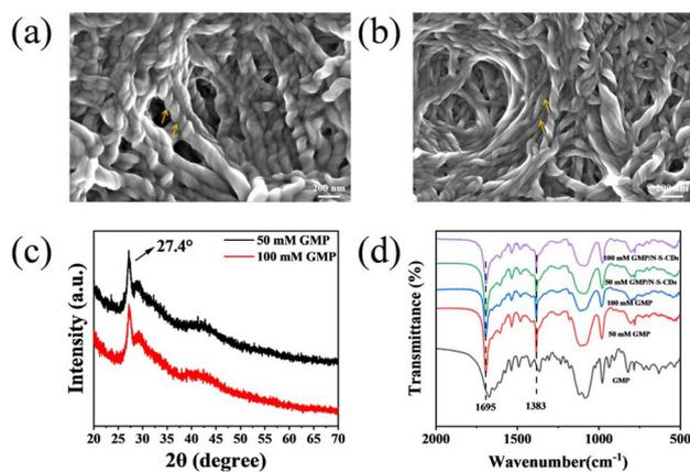
**Fig. 3** (a) SEM images of the right-handed N-S-CDs/g-fiber and (b) left-handed N-S-CDs/g-fiber; (c) XRD and (d) FTIR spectra of GMP, right-handed g-fiber, left-handed g-fiber, and N-S-CDs/g-fiber composites.
