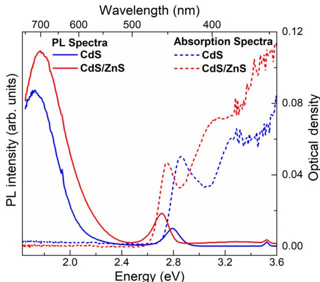
Fig. 2 Optical absorption (dashed lines) and PL emission (solid lines) spectra of interface-engineered CdS QDs are shown in blue. Those spectra of the same batch of CdS QDs after overcoating with ZnS shell are shown in red.
