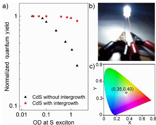
**Fig. 5** (a) The normalized quantum yield of CdS QDs without and with intergrowth phases as a function of optical density (OD) at S exciton. (b) Prototype device, emitting white light after coating a UV LED with 3.0 nm diameter CdS quantum dots with designed intergrowth phases embedded in PMMA. (c) Coordinate in CIE diagram shows that emission from this CdS-coated LED is in the white region.
