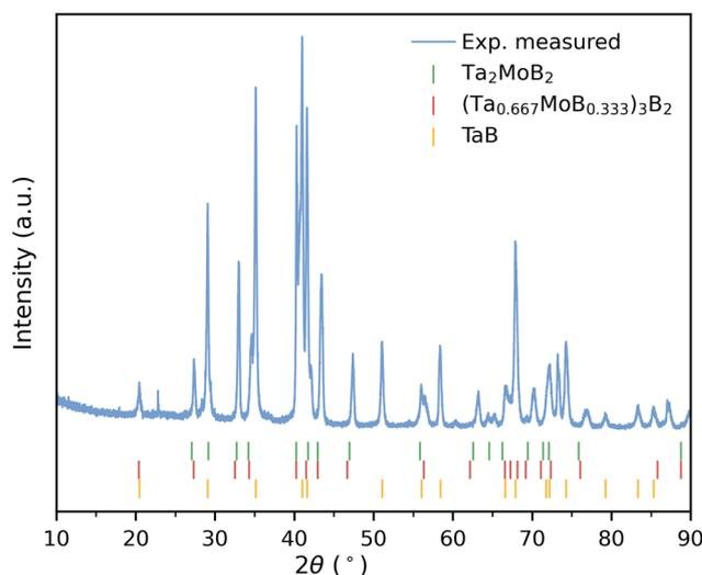
**Fig. 4** XRD pattern of the sample from the attempted synthesis of  $Ta_2MoB_2$  with assigned peaks for  $Ta_2MoB_2$ ,  $(Ta_{0.667}Mo_{0.333})_3B_2$ , and TaB, given by green, red, and yellow vertical bars respectively.
