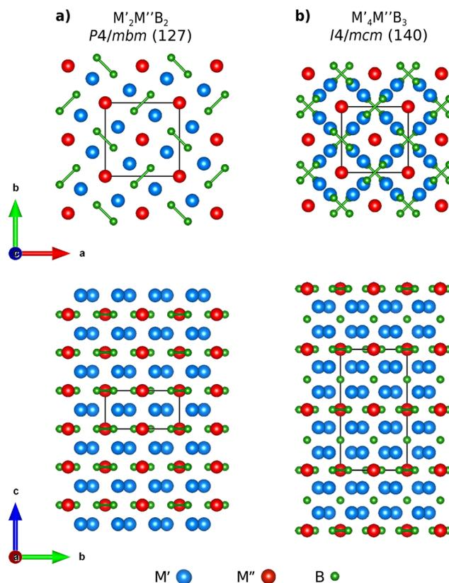
**Fig. 1** Schematic illustration of (a)  $M'_2M''B_2$  ( $P4/mbm$ ) and (b)  $M'_4M''B_3$  ( $I4/mcm$ ) along the  $[001]$  and  $[100]$  zone axes, with atoms of the two metal sites represented by blue and red while boron atoms are in green.
