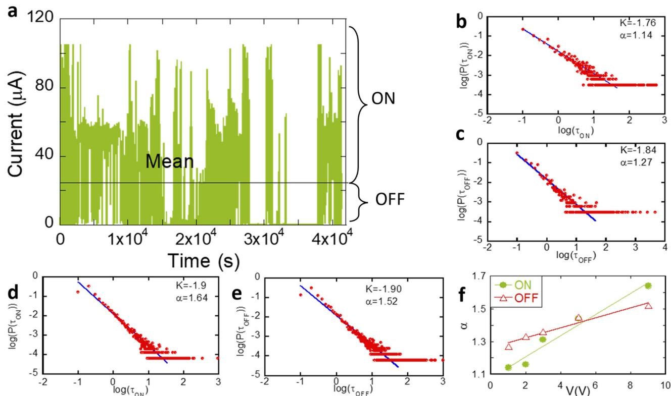
**Fig. 4** (a) Variation of current at 1 V at the LRS; (b and c) power law analysis of ON and OFF times, respectively, at 1 V; (d and e) power law analysis of ON and OFF times at 9 V, respectively; and (f) variation of  $\alpha$  with bias voltage.
