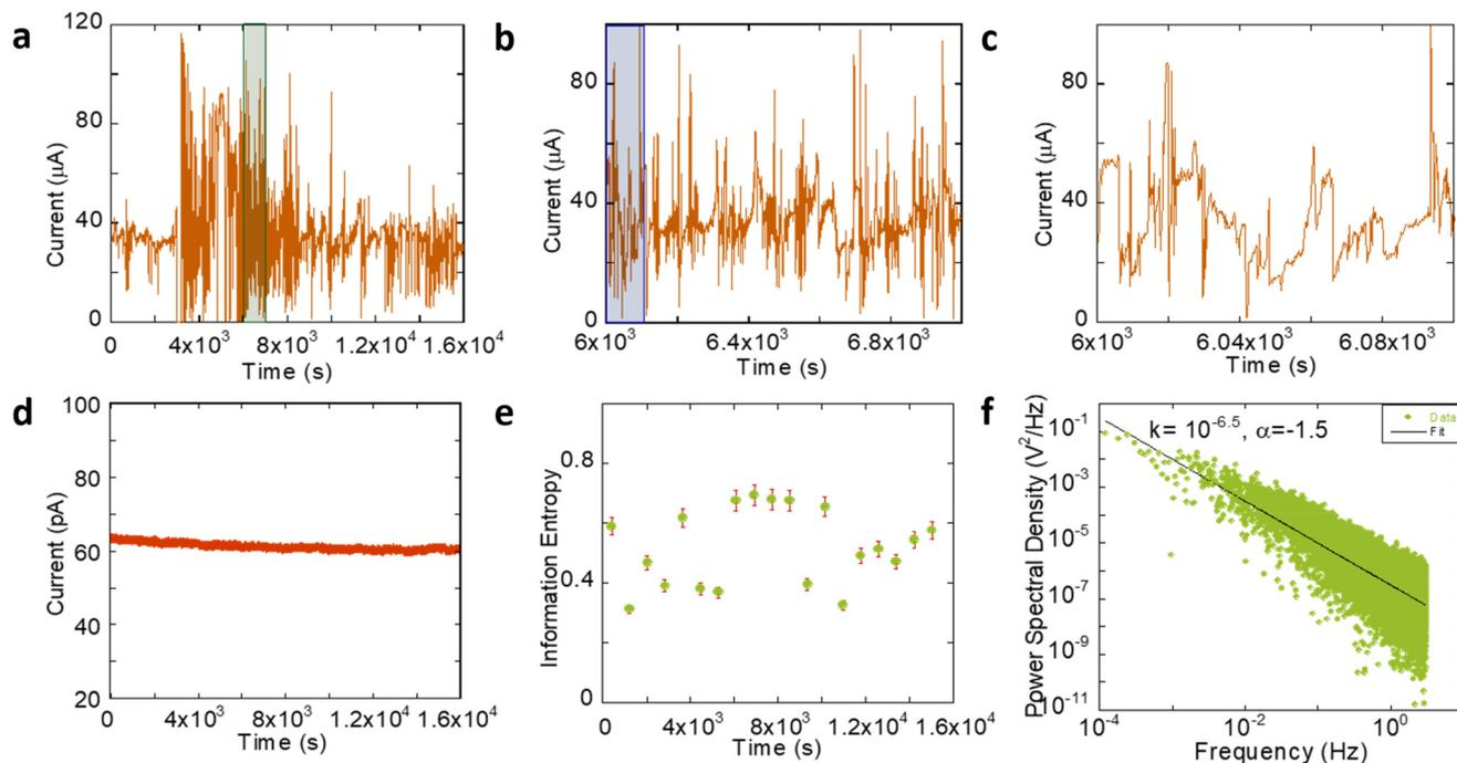
**Fig. 3** (a–c) Variation of current over three different time ranges during the LRS taken at fixed 1 V bias; (d) fluctuation of current over time at the HRS at 1 V bias; (e) information entropy derived from a; and (f) Fourier transform of a.
