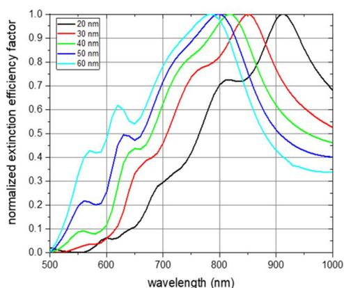
**Fig. 4** Simulation results of the optical extinction efficiency factor for varying nanoparticle thicknesses in dependence of the wavelength. Nanoparticle thickness of 20 nm is shown in black, 30 nm in red, 40 nm in green, 50 nm in blue, and 60 nm in cyan. Nanoparticles are oriented randomly, the excitation light is unpolarized, and the extinction efficiency factors are normalized.
