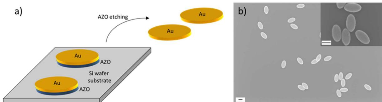
**Fig. 3** Sketch of the nanoparticle transfer to solution and SEM images of the nanoparticles. (a) Sketch of gold (Au) nanoparticle transfer from the silicon wafer substrate to solution *via* etching of the sacrificial aluminium-doped zinc oxide (AZO) layer. (b) SEM images of the nanoparticles after drop-casting from solution onto an imaging substrate. Overview at lower magnification and detailed image at higher magnification (inset in the top right). The scale bars correspond to 200 nm.
