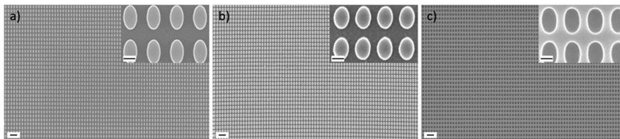
**Fig. 2** Scanning electron microscopy (SEM) images. Overview at lower magnification and detailed image at higher magnification (inset in the top right). (a) Si master stamp. (b) Polydimethylsiloxane (PDMS) stamp. (c) UV-NIL imprinted nanostructure. The scale bars correspond to 1  $\mu\text{m}$  for the large overview images and to 200 nm for the insets showing details at higher magnification.
