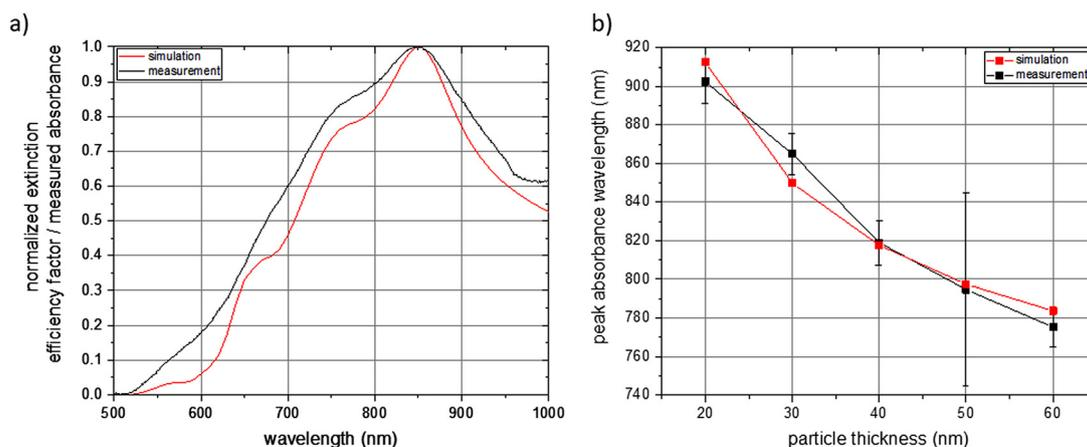
**Fig. 5** Comparison of the simulated (red line) and measured (black line) absorbance spectrum. (a) Normalized simulated and measured spectra for a nanoparticle with 30 nm thickness. (b) Peak absorbance wavelengths in dependence of the nanoparticle thickness. For both images, the nanoparticles are oriented randomly, and the excitation light is unpolarized for the simulation as well as for the measurement.
