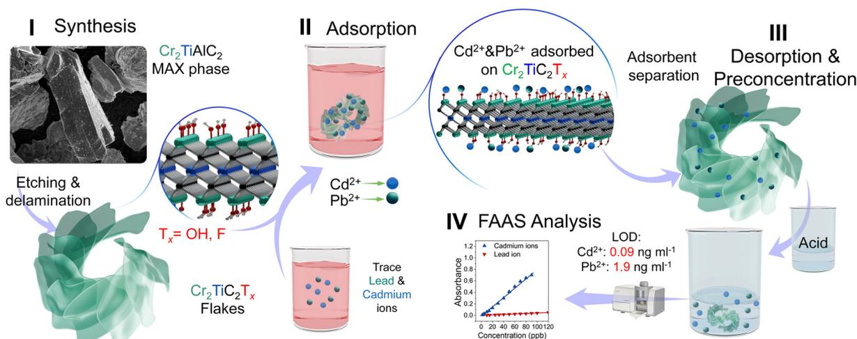
**Scheme 1** Schematic illustration of the application of  $\text{Cr}_2\text{TiC}_2\text{T}_x$  MXene as a solid phase in ultrasonic-assisted d- $\mu$ -SPE for heavy metal detection.
