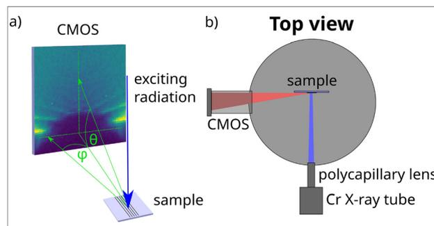
**Fig. 2** (a) Schematic drawing of the setup geometry with the emission angles  $\theta$  and  $\varphi$ . (b) Schematic top view of the setup. The UHV chamber with the sample inside is shown as well as the Cr X-ray tube with the polycapillary lens to focus the radiation as well as the Tucson Dhyana 95 CMOS detector. The CMOS is mounted on the outside of the UHV chamber via an adapter flange.
