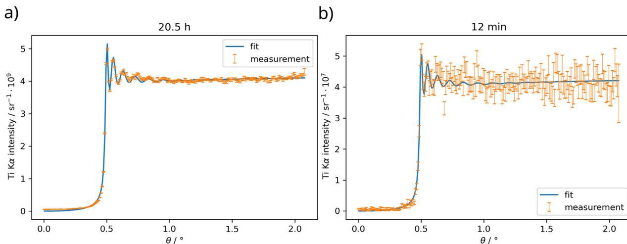
**Fig. 3** (a) Measured angle-dependent Ti K $\alpha$  fluorescence emission profile of the layered sample in orange with the full data of 20.5 h measurement time. The error bars depict the statistical uncertainties originating from the total photon counts of each emission angle. (b) The same measurement utilizing only the first 12 min of the full data set and the respective fit.
