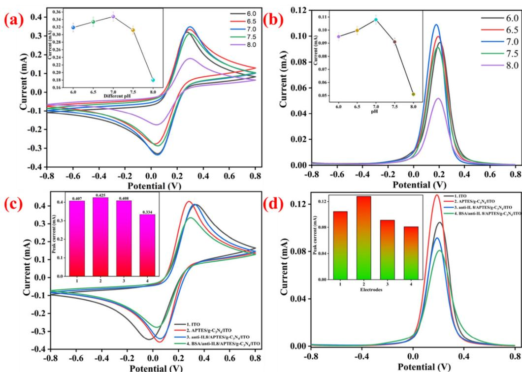
**Fig. 6** pH study using (a) CV and (b) DPV techniques (the line plot demonstrating the correlation between the pH and the peak current (oxidation) can be found in the inset images); (c) CV and (d) DPV curves of various modified electrodes (the bar plot between the peak current and various modified electrodes is displayed in the inset). Three distinct experiments were conducted to acquire the error bars.
