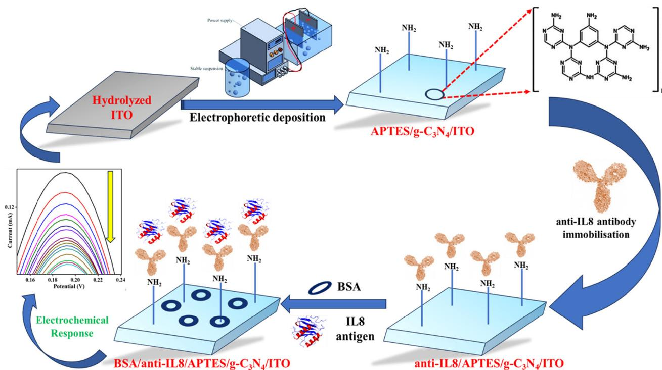
**Scheme 2** An illustrative diagram outlining the sequential process of creating an immunoassay platform to detect the IL8 biomarker in saliva samples utilizing *g*-C<sub>3</sub>N<sub>4</sub> as the foundation.
