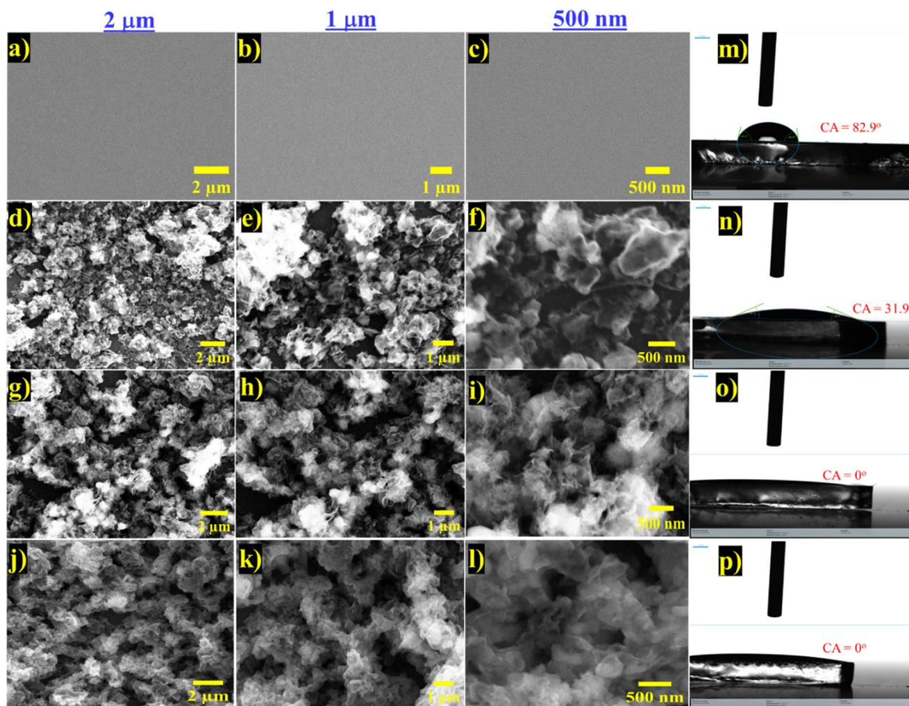
Fig. 4 SEM images at 3 different scales, *i.e.*, 2  $\mu\text{m}$ , 1  $\mu\text{m}$ , and 500 nm of each modified electrode: (a–c) ITO, (d–f) APTES@g-C<sub>3</sub>N<sub>4</sub>/ITO, (g–i) anti-IL8/APTES@g-C<sub>3</sub>N<sub>4</sub>/ITO, and (j–l) BSA/anti-IL8/APTES@g-C<sub>3</sub>N<sub>4</sub>/ITO; contact angle studies of (m) ITO, (n) APTES@g-C<sub>3</sub>N<sub>4</sub>/ITO, (o) anti-IL8/APTES@g-C<sub>3</sub>N<sub>4</sub>/ITO, and (p) BSA/anti-IL8/APTES@g-C<sub>3</sub>N<sub>4</sub>/ITO.
