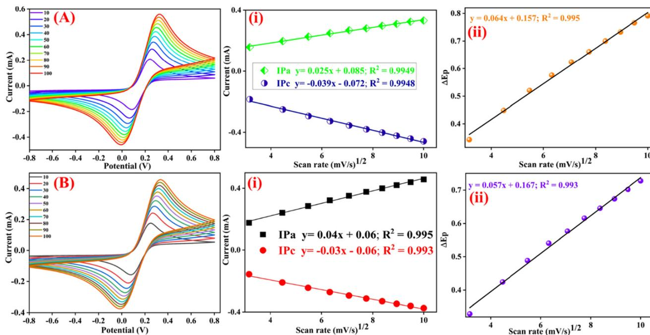
**Fig. 5** CV profiles of (A) the APTES@g-C<sub>3</sub>N<sub>4</sub>/ITO electrode and (B) the BSA/anti-IL8/APTES@g-C<sub>3</sub>N<sub>4</sub>/ITO immunoelectrode. (A(ii)) and (B(ii)) display the oxidation and reduction peak currents normalized to the square root of the scan rate, while (A(ii)) and (B(ii)) demonstrate the divergence observed in cathodic and anodic peak potentials ( $\Delta E_p$ ) in relation to the square root of the scan rate.
