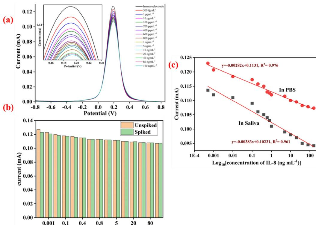
**Fig. 9** (a) The constructed immunoelectrode showing the electrochemical DPV responses when IL8 concentrations ranging from 500 fg mL<sup>-1</sup> to 160 ng mL<sup>-1</sup> are added in the presence of actual samples; (b) a comparison between the fabricated biosensor current response in the standard and spiked samples; and (c) a calibration curve graph created between the peak current and the IL8 concentrations using both real and standard samples.
