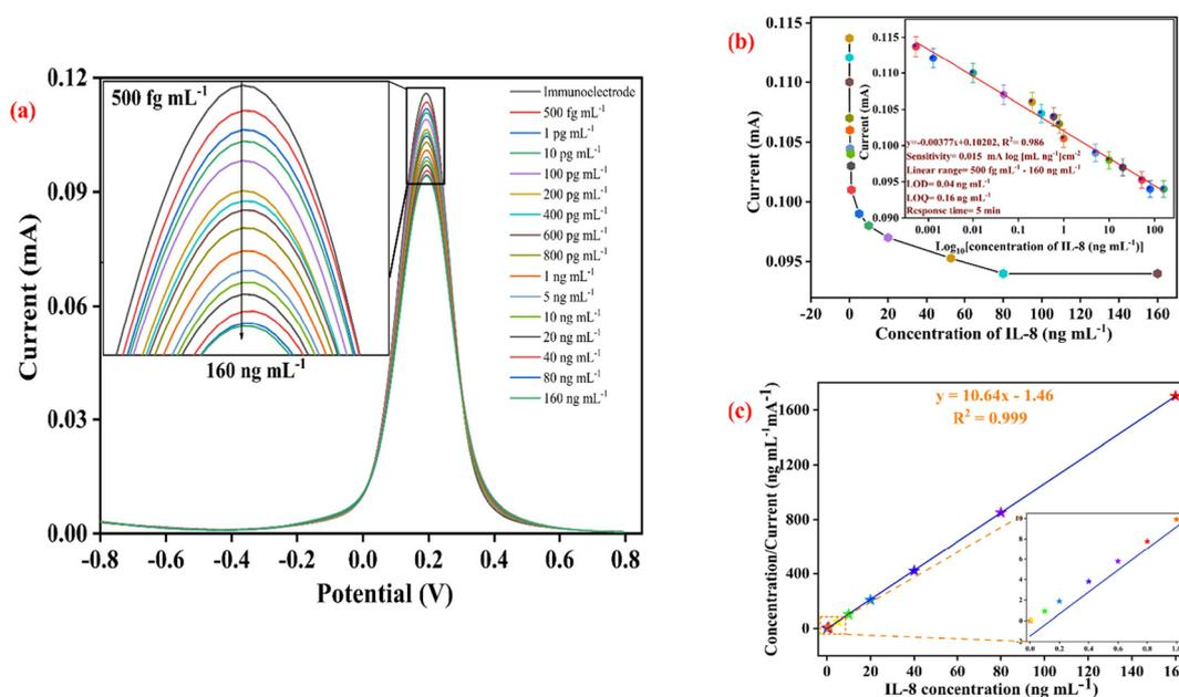
**Fig. 7** (a) Illustration of the electrochemical response of the sensing platform towards IL8 concentrations using DPV (the enlarged view is displayed in the inset); (b) a calibration plot obtained using DPV techniques between the anodic peak current magnitude and the  $\log_{10}$  of the IL8 concentration; and (c) Hanes–Wolf plot. Three separate tests were conducted to acquire the error bars.
