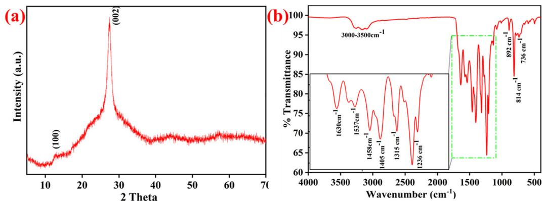
Fig. 1 (a) XRD patterns and (b) FT-IR spectra of g-C<sub>3</sub>N<sub>4</sub>.
