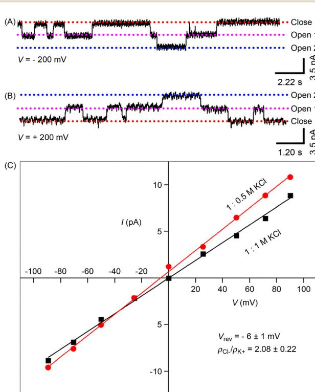
**Fig. 3** Current traces recorded with **1d** (*c* = 2.0 μM) at –200 mV (A) and +200 mV (B) in a symmetrical KCl solution. Current–voltage relationship of **1d** in both symmetrical and asymmetrical KCl concentrations (C).
