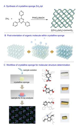
Fig. 1 Fujita's crystalline sponge for molecular structure determination. Reprinted with permission from ref. 7. Copyright 2013 Springer Nature Limited
