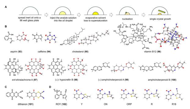
Fig. 6 ENaCt for structure elucidation of organic molecules. (A) The workflow and principle of ENaCt method. (B-D) Chemical and crystal structures of organic molecules elucidated by ENaCt.
