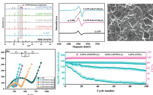
**Effect of Sb<sup>3+</sup> doping on the electrochemical performance of a LATP solid electrolyte**
