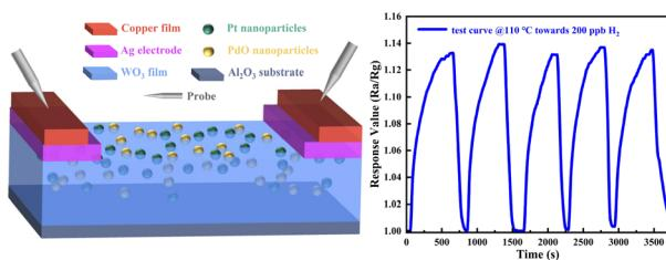
**A high-performance H<sub>2</sub> gas sensor based on PtO<sub>x</sub> and PdO<sub>y</sub> co-decorating WO<sub>3</sub> film**
