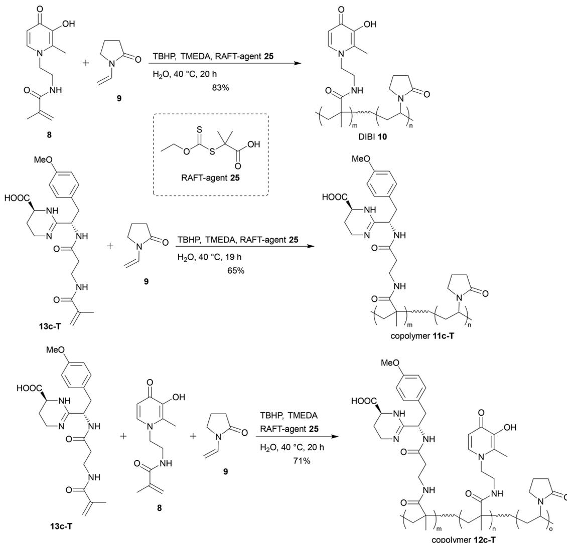
**Scheme 4** Polymerization conditions towards DIBI **10** and methyl-protected **13c-T** with NVP (**9**), MAHMP (**8**), RAFT-agent (**25**), tetramethylethylenediamine (TMEDA) and *tert*-butyl hydroperoxide (TBHP).
