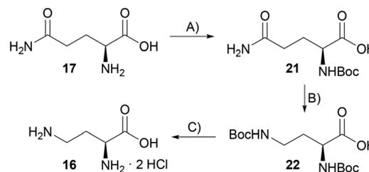
**Scheme 2** Synthesis of DABA **16**. (A)  $\text{Boc}_2\text{O}$ , NaOH,  $\text{H}_2\text{O}$ , THF, rt, 22 h, 67%; (B)  $\text{Br}_2$ , NaOH,  $\text{H}_2\text{O}$ , 0 °C to 80 °C, 2 h, then  $\text{Boc}_2\text{O}$ , NaOH,  $\text{H}_2\text{O}$ , 1,4-dioxane, rt, 24 h, 44%; (C) concentrated HCl, rt, 2 h, 84%.
