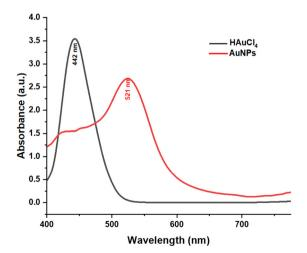
Fig. 2 LSPR absorption spectrum of hydrogen tetrachloroaurate (gold ions) and gold nanoparticles
