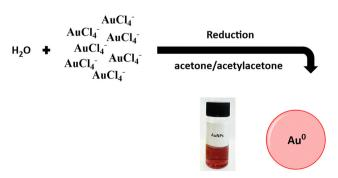
Scheme 1 Schematic representation of the synthesis of gold nanoparticles during the process.
