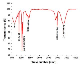
Fig. 4 FTIR spectra of gold nanoparticles.
