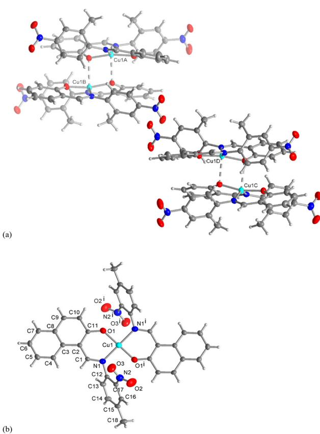
**Fig. 7** Molecular structures of compounds (a) **1** and (b) **3** (50% thermal ellipsoids and H atoms with arbitrary radii). The asymmetric unit of **1** in (a) depicts the two symmetry-independent dinuclear pairs with the four  $\text{Cu}(\text{L}^1)_2$  moieties (denoted as A, B, C, D; see Fig. S10 and S11 for full atom labelling). The dashed lines indicate the long Cu–O bonds of around 2.5 Å. Symmetry transformation in (b) **3**:  $i = 2 - x, 1 - y, 1 - z$ .
