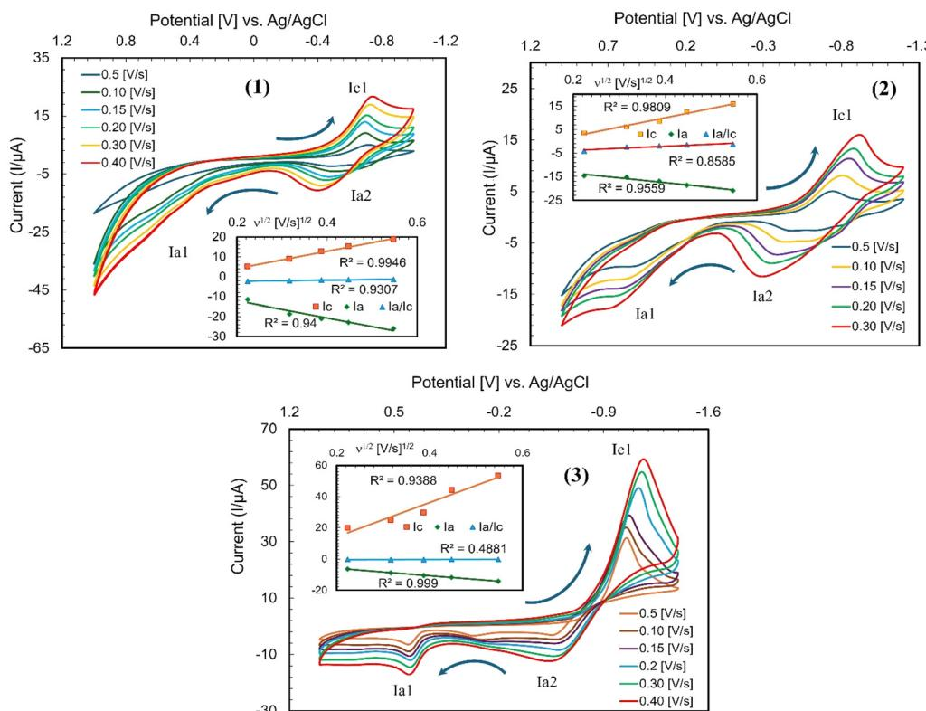
Fig. 10 CV patterns for complexes **1**, **2** and **3** (ca. 0.5 mmol L<sup>-1</sup>) at varying scan rates (v/V s<sup>-1</sup>) in DMF at 25 °C; supporting electrolyte: tetra-N-butylammonium hexafluorophosphate (TBAP) (ca. 0.1 mol L<sup>-1</sup>); inset: plot of peak current (Ic1 or Ia1) vs. square root of the scan rate ( $v^{1/2}$ ).
