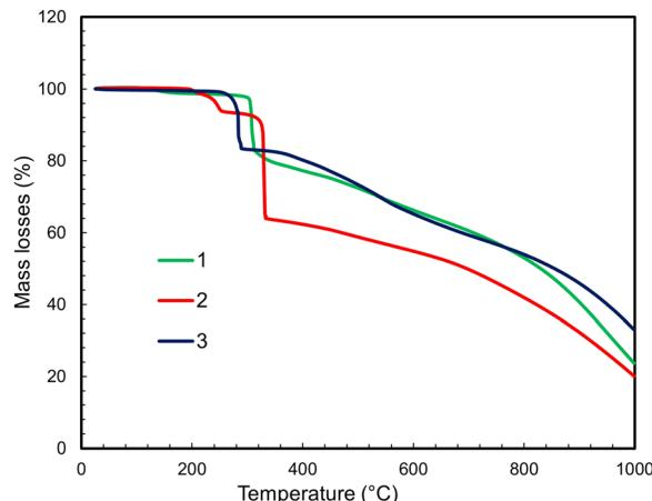
Fig. 5 Thermogravimetric analysis (TGA) curves of complexes **1**, **2** and **3** (a heating rate of 5 K min<sup>-1</sup> under an N<sub>2</sub> atmosphere).
