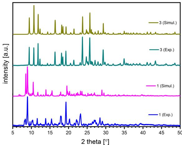
**Fig. 9** Experimental and simulated (from single-crystal X-ray structure) PXRD patterns for the copper complexes **1** and **3**. The experimental PXRD patterns were collected at ambient temperature, and the underlying crystal structures used for the simulations were obtained at 150 K (**1**) and 299 K (**3**).
