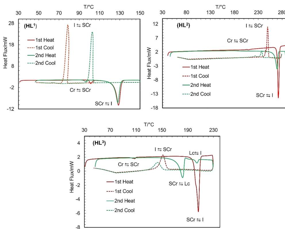
Fig. 4 Differential scanning calorimetry (DSC) analyses for the Schiff base ligands.
